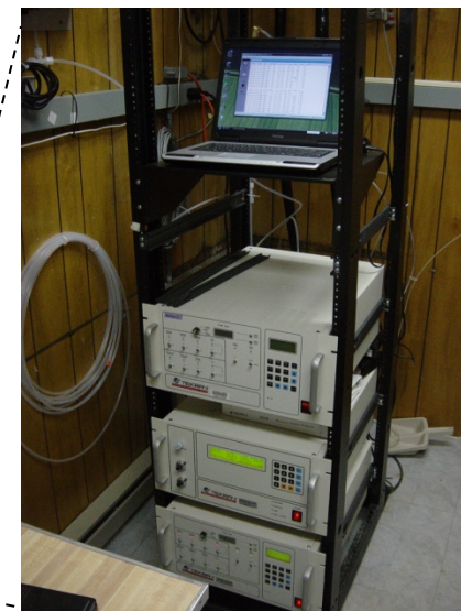
After RGM and Hg(p) is collected, it is desorbed and analyzed inside the trailer, along with Hg(0)
