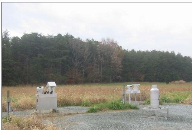
Precipitation measurements (left to right): Mercury Deposition Network, Major Ions (e.g. "acid rain"), Precipitation Amount
