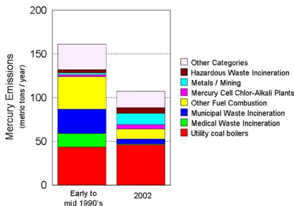
Fig. 1. Estimated US anthropogenic mercury emissions in the early-to-mid 1990s and 2002. As described in the methodology section, the estimates for the earlier period are based on US EPA data as described in Cohen et al. (2004) and the 2002 estimates are based on the US EPA 2002 National Emissions Inventory (US EPA, 2007).
