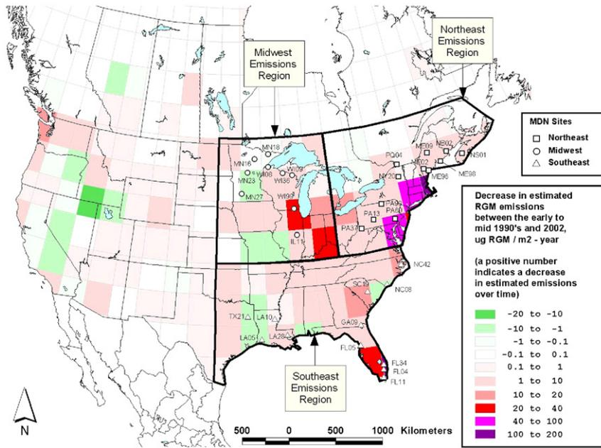
Fig. 3. MDN sites/regions analyzed and reactive gaseous mercury (RGM) emissions flux changes between the early-to-mid 1990s and 2002. The emissions inventories described herein were allocated to a  $3^\circ \times 3^\circ$  grid to produce the geographical distribution of RGM changes shown.
