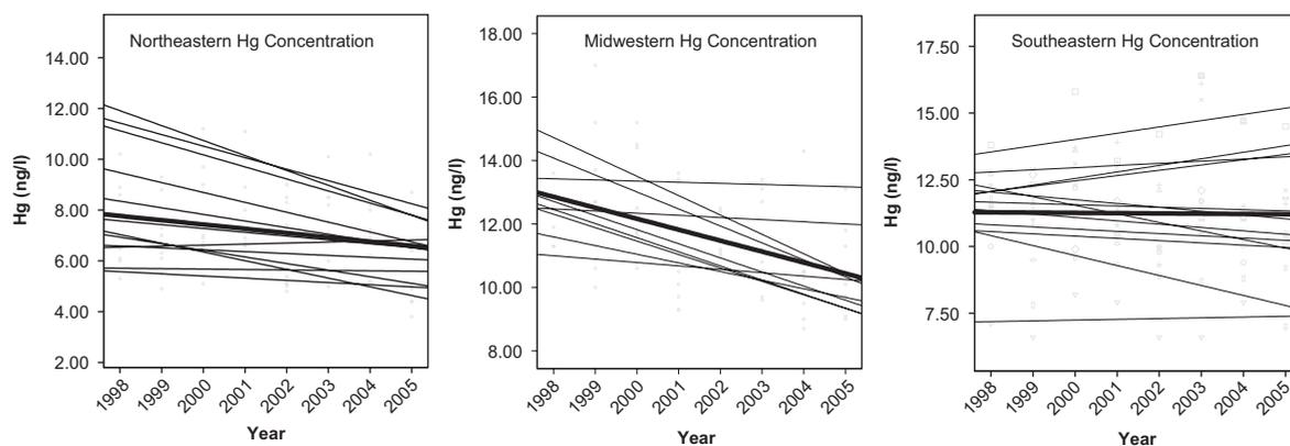
Fig. 6. Random coefficient model results for the relation between time and annual volume-weighted concentration measured at MDN sites for the Northeastern (NE), Midwestern (MW), and Southeastern (SE) USA for 1998–2005. The bold line in each graph represents the overall regression line for the region. The other lines are regressions for each site in the region.
