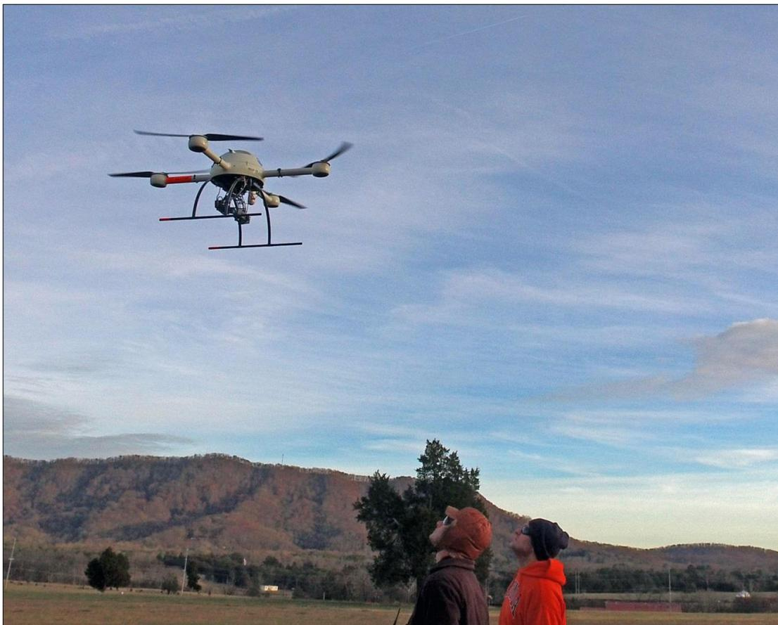
**Figure 2: The Microdrone MD4-1000 flying at House Mountain Radio Control (HMRC), Corryton, TN.**
