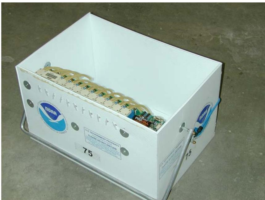
Figure 17. Bag sampler with cover and cartridge removed.
