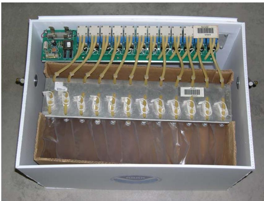
Figure 19. Bag sampler with sampler cartridge installed.
