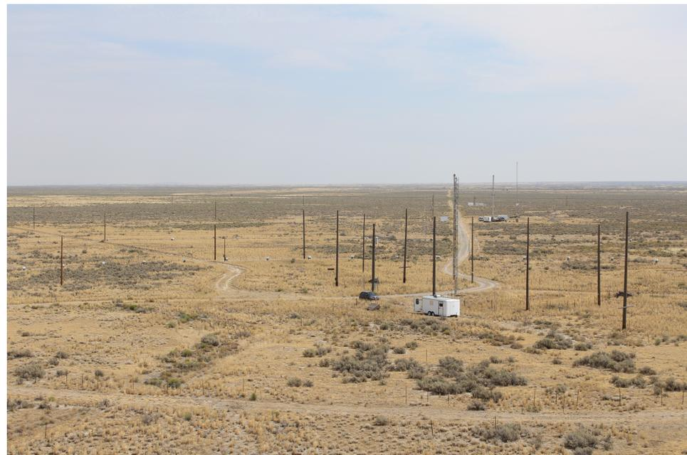
Figure 3. Photo from Grid 3 tower looking northeast along the radial road at 55° azimuth through the tracer sampling array. The release site is near the center of the photo, the command center (COC) tower and wind profiler installation (PRO) are visible in the right center of the photo, and the ridge to the northeast of the release is visible in the upper left.
