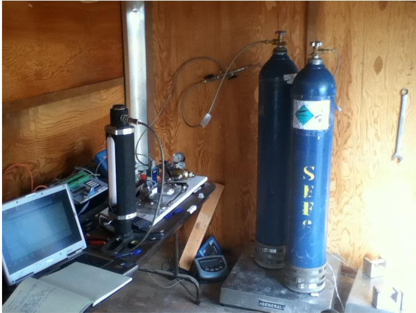
Figure 7. The SF<sub>6</sub> release system inside the cargo trailer including the SF<sub>6</sub> bottles, mass flow controller, computer data acquisition and control system, and electronic scales under the bottles.
