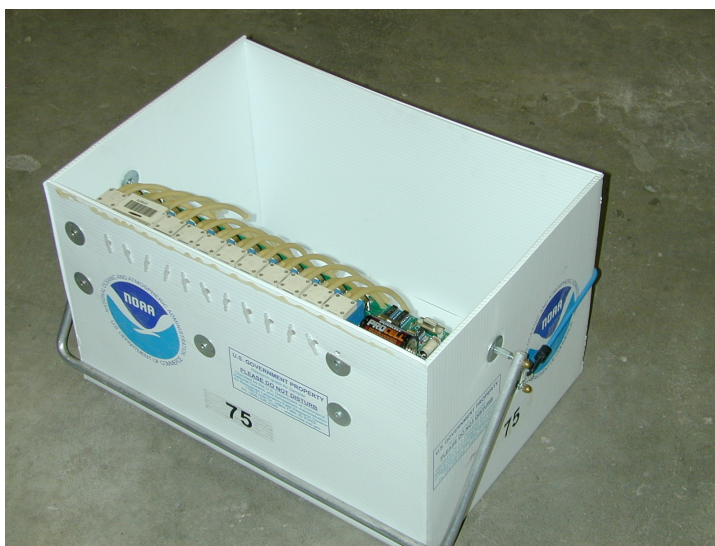
Figure 18. Bag sampler with cover and cartridge removed.
