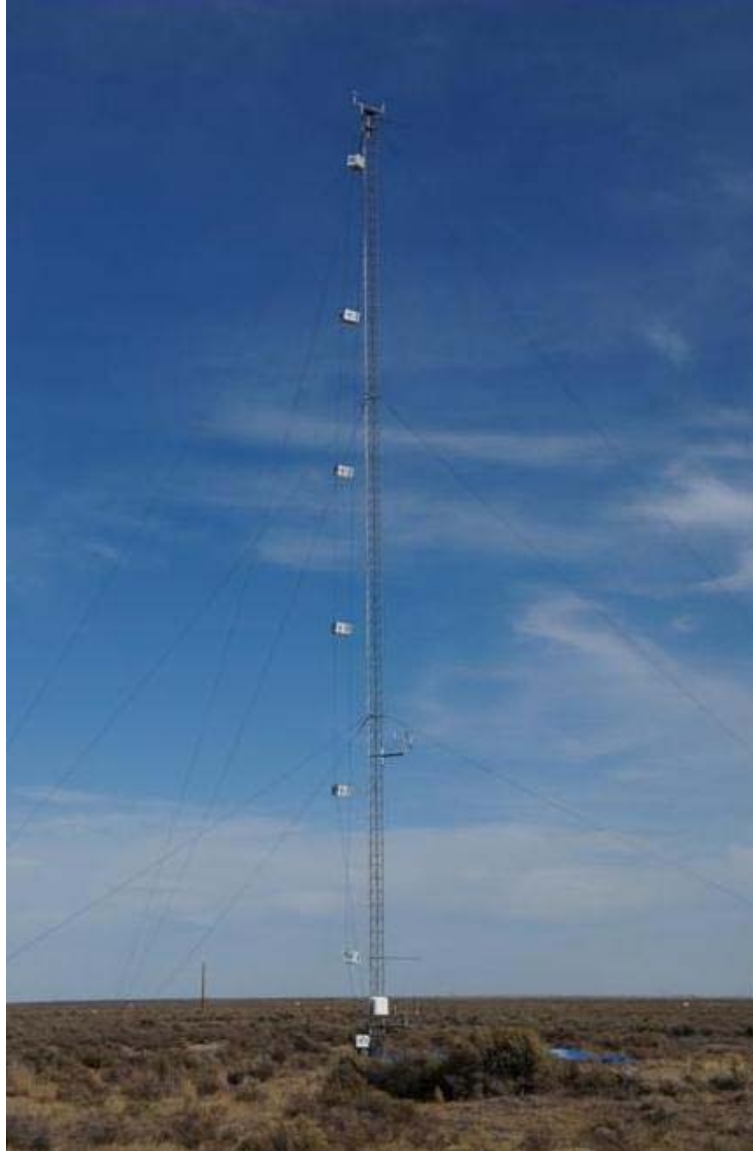
Figure 53. 30 m command center meteorological and tracer sampling tower (COC).
