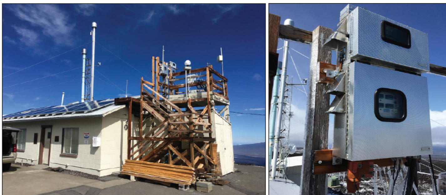
MLO. Left: ARL's instruments reside on the exterior platform of the historic Keeling Building. Right: A close-up of the atmospheric mercury measurement equipment shows the particulate-bound mercury and gaseous oxidized mercury monitors (top and bottom boxes, respectively). Credit: NOAA
