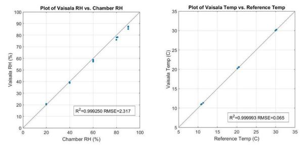
Results shown above: A plot of the reference temperature versus Vaisala temperature (left), and a plot of the reference humidity versus Vaisala humidity (right). The R2 values are 0.999993 and 0.999250 for the temperature and relative humidity, respectively. The reference instrument for the temperature was a Hart Scientific platinum resistance thermometer (PRT), while the reference for the humidity was the Thunder Scientific chamber itself.
