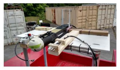
Four channels were tested for each sensor: Air temperature, Humidity, Air pressure, and Infrared (sea) temperature. Ground speed was also measured and recorded.
