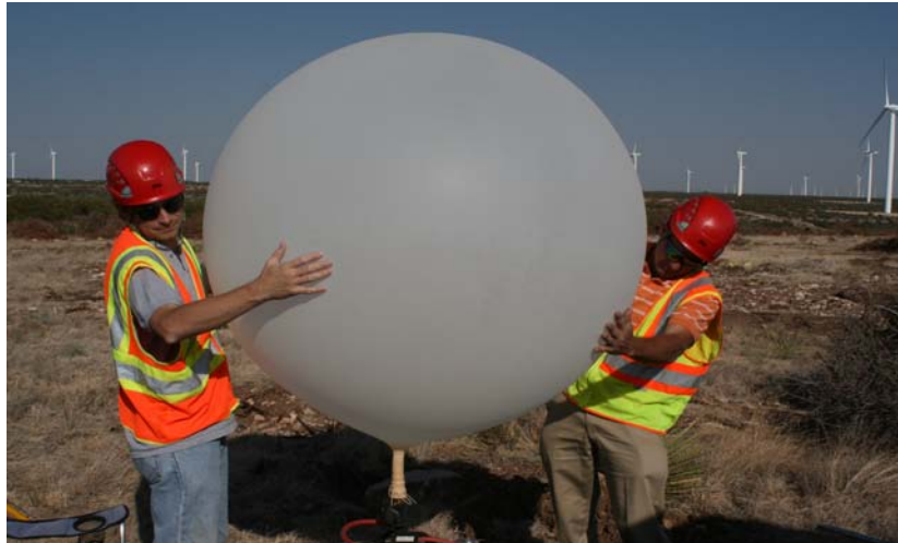
Ed Dumas (left) and Randy White (right), with ARL's Atmospheric Turbulence and Diffusion Division, inflate a weather balloon as part of the Texas radiosonde study.
