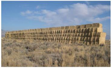
length, constructed of 300 1-ton straw bales, has been built at the Grid 3 facility on the INL (Fig. 1). Pollutant transport and dispersion will be measured in field tests using the atmospheric tracer sulfur
