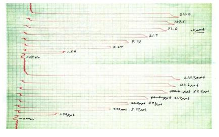
sensitive to the humidity of the sample stream so that drying of the sample gas will be essential. It is apparent that an oxygen/water removal system similar to the existing fast response analyzers will be needed with this detector and several options are under consideration. Although there are obstacles to overcome, the project looks promising. <u>roger.carter@noaa.gov</u>, Shane Beard, and Randy Johnson
