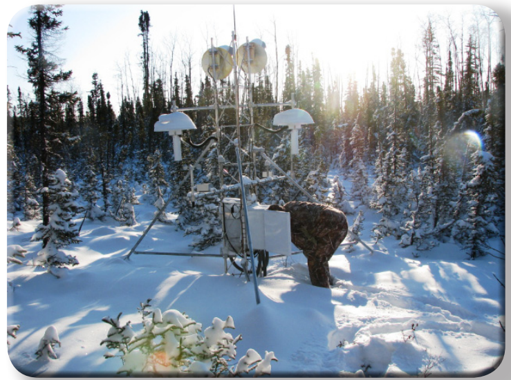
A recent U.S. Climate Reference Network station, installed by ARL in the Tetlin National Wildlife Refuge near Tok, AK, is powered by new fuel cell technology. The station provides high-quality, long-term climate observations of temperature and precipitation in one of the coldest regions below the Arctic Circle. On 1/21/12 temperatures dipped to -51 °F. Photo: NOAA
