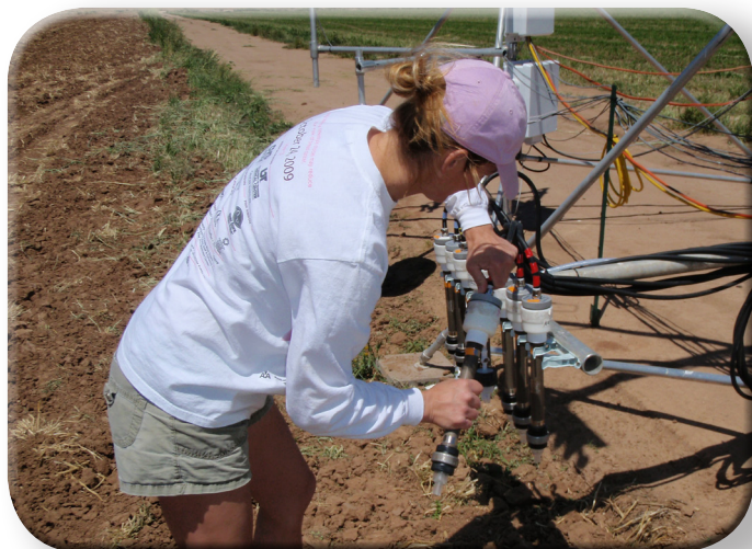
ARL technician collecting ammonia measurements over an agriculture field during a major California air quality study in 2010. Photo: NOAA
