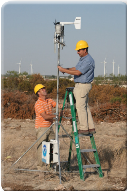
ARL scientists gearing up to collect atmospheric measurements in the vicinity of wind turbines in West Texas. The data collected and analyzed by ARL will improve forecasts of winds at heights more relevant to the wind energy industry. Photo: NOAA
