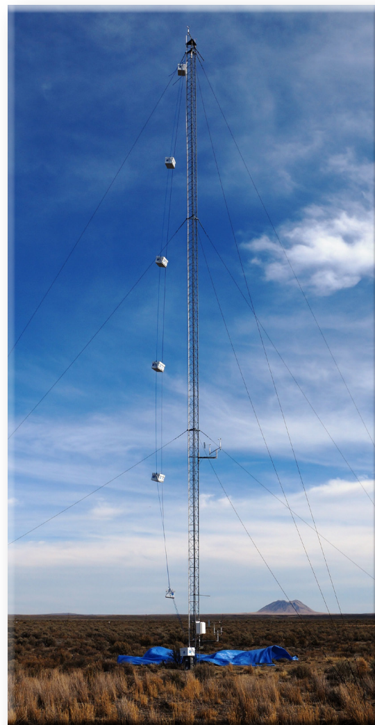
A NOAA/INL tower containing meteorological instrumentation and atmospheric tracer technology for a multi-year research study called "Project Sagebrush." To improve dispersion models, this study is re-evaluating atmospheric dispersion studies conducted during the 1950s but with modern instrumentation and technologies. Photo: NOAA
