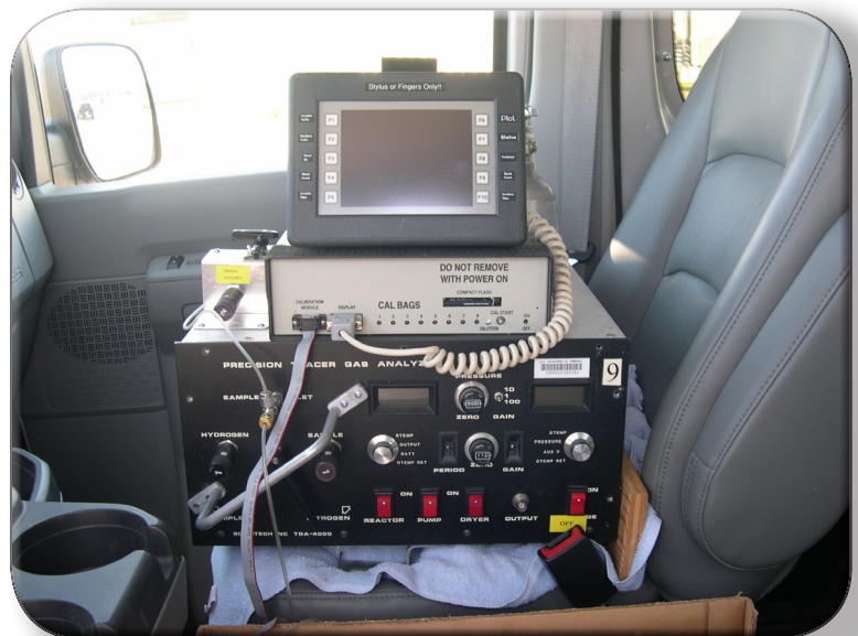
A fast response analyzer that measures tracer concentrations every second. The analyzer is easily carried on a seat of a vehicle. Photo: NOAA/ARL
