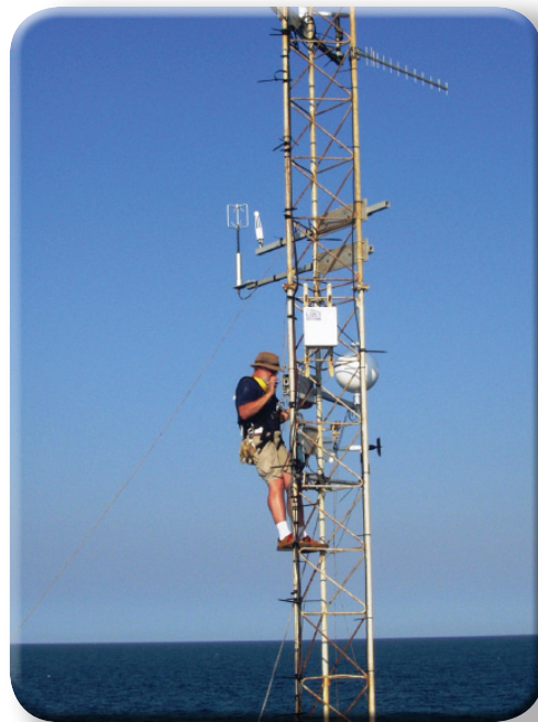
ARL scientist deploying an ET Probe on a tower at the end of a 560 meter long pier in Duck, NC Image: NOAA.
