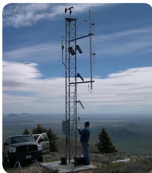
ARL performs routine maintenance at one of the high-resolution meteorological stations located at the top of Big Southern Butte in Idaho. Photo: NOAA
