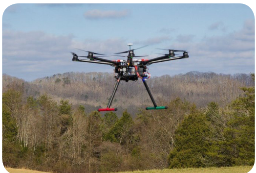
The ARL sUAS in a test flight at the Knox County Radio Control Society's model flying field near Knoxville, TN. The sUAS collects boundary layer measurements. Photo: NOAA
