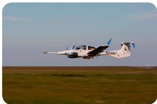
The ARL BAT probe positioned on the nose of the Centaur aircraft to measure turbulence in the boundary layer. Photo: NOAA
