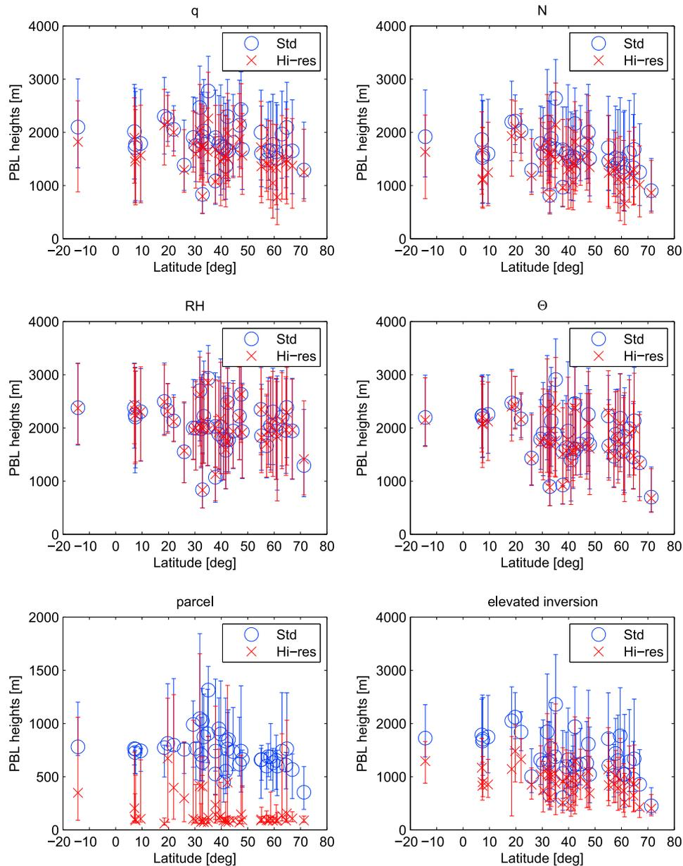
**Figure 10.** Comparison of 25th, 50th and 75th percentile values of PBL heights (m) from 44 stations based on standard (blue) and high (red) vertical resolution sounding data, as a function of station latitude. Each frame shows results for a different method of estimating PBL height using observations for 1999–2007. Note the different vertical axis scale for the parcel method (lower left frame).
