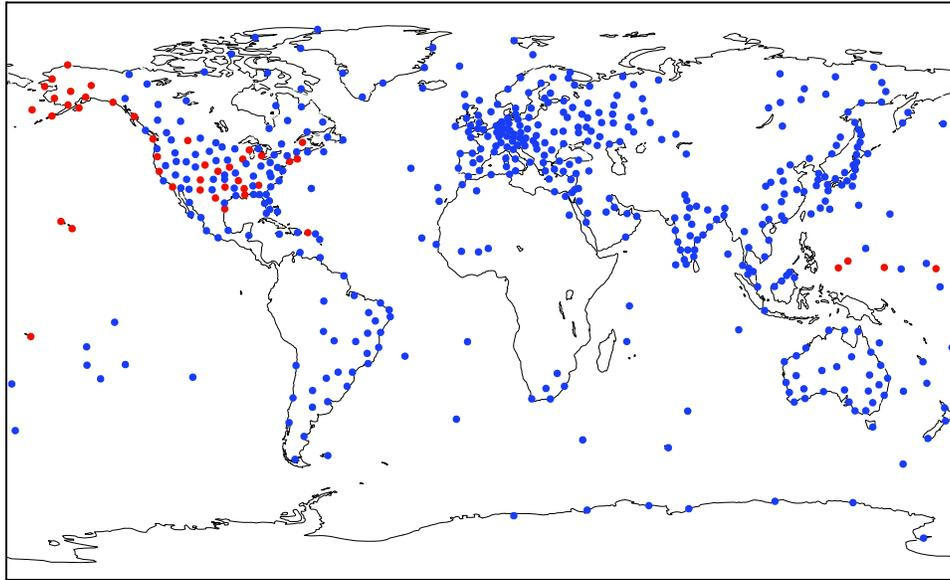
**Figure 1.** Map of 505 radiosonde stations used in this study. The 44 U.S.-operated stations shown in red have high-vertical-resolution observations and were used to analyze the effect of vertical resolution on estimated PBL height.
