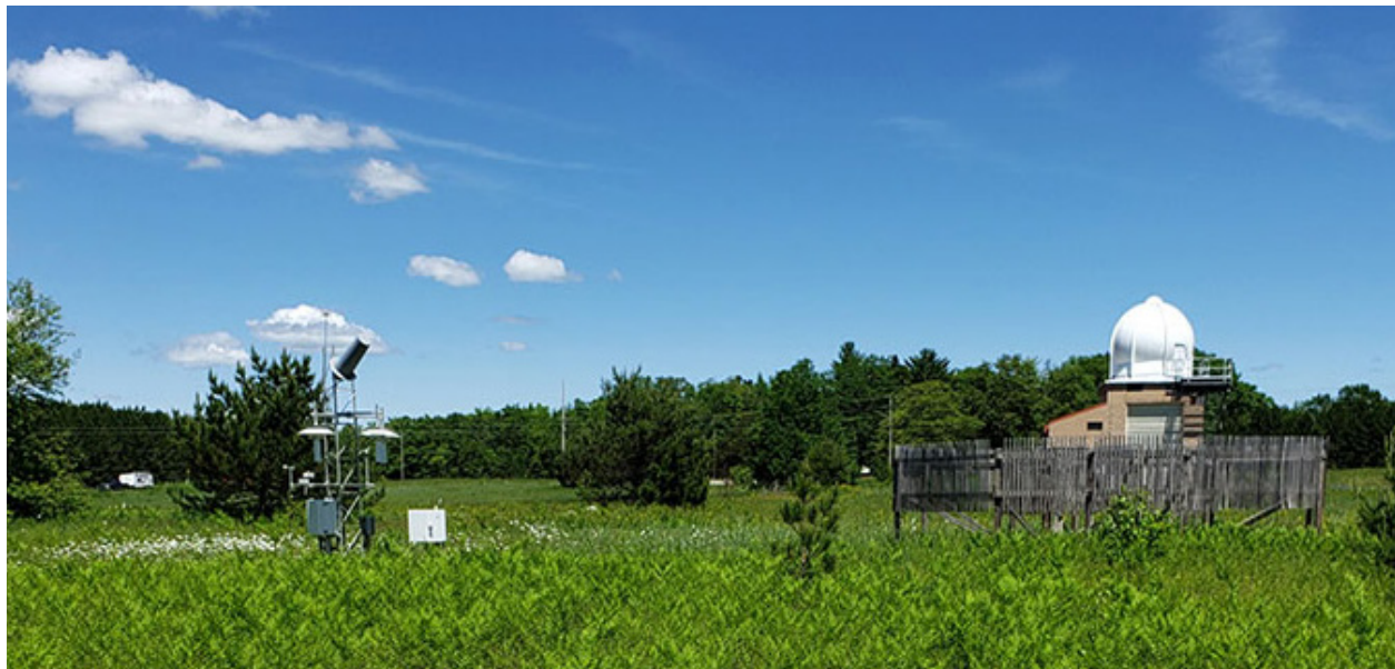
US Climate Reference Network Station in Gaylord, Michigan. The precipitation gauge at right, is surrounded by fencing. Image credit: NOAA
