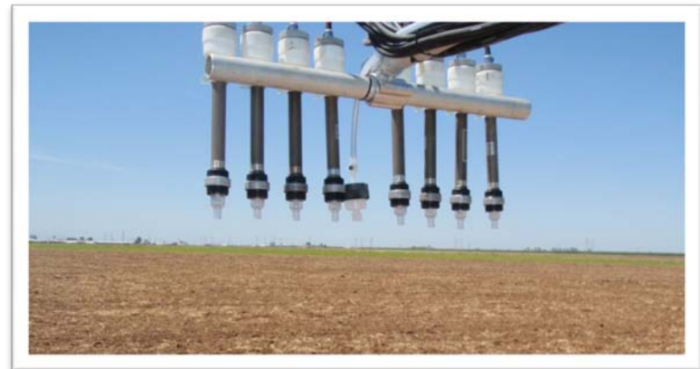
Fast-response sensor (inlet shown center) and traditional annular denuder samplers in California.
