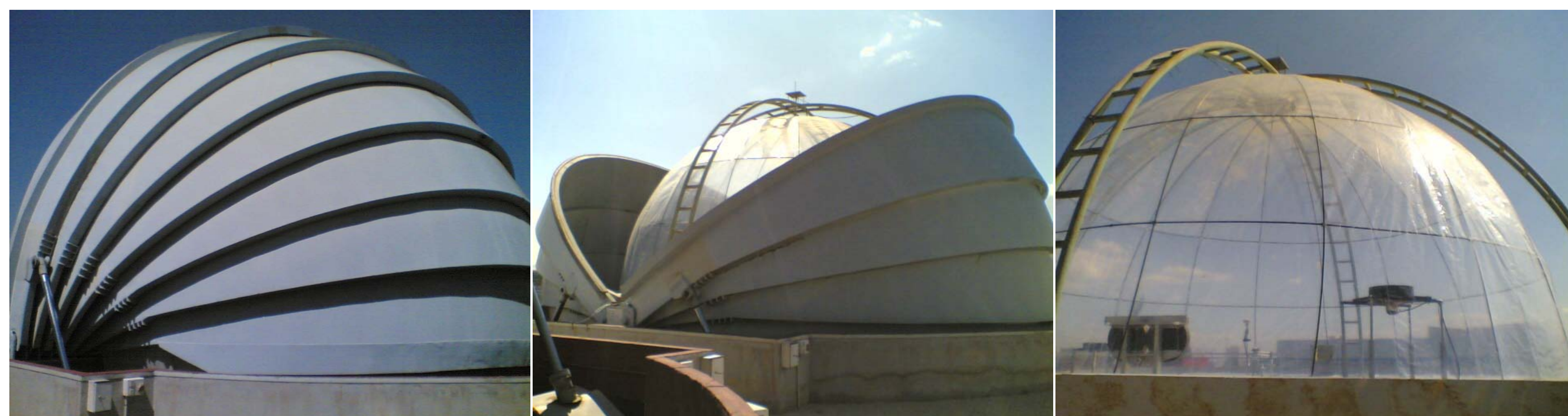
FIGURE 1. EUPHORE CHAMBER (CEAM, Valencia, SPAIN). As the chamber opens to the sunlight, the photochemical oxidation of the VOCs starts
