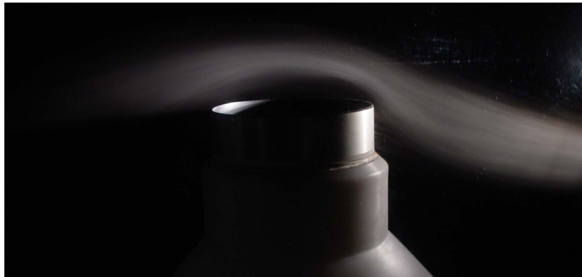
Figure 1. Air flow over a precipitation gauge within the Atmospheric Turbulence and Diffusion Division wind tunnel.
