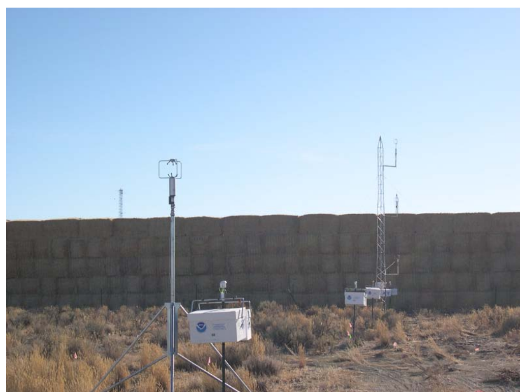
Figure 4. Vertical profile tower behind tower with bag samplers hanging on fence posts.
