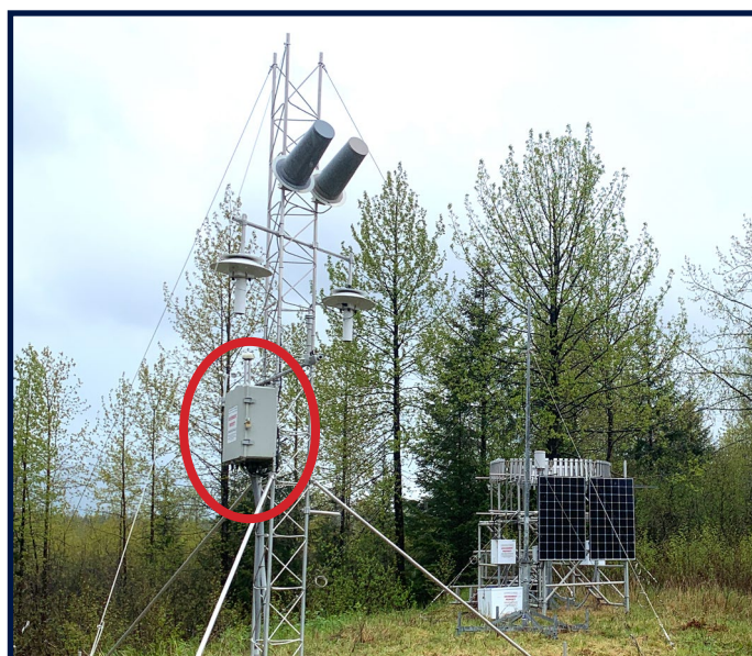
USCRN station in Cordova, AK. Red circle designates the data logger box where the new transmitters are located. Credit: Chuck Lindsay (Williwaw Weather and Climate Services)
