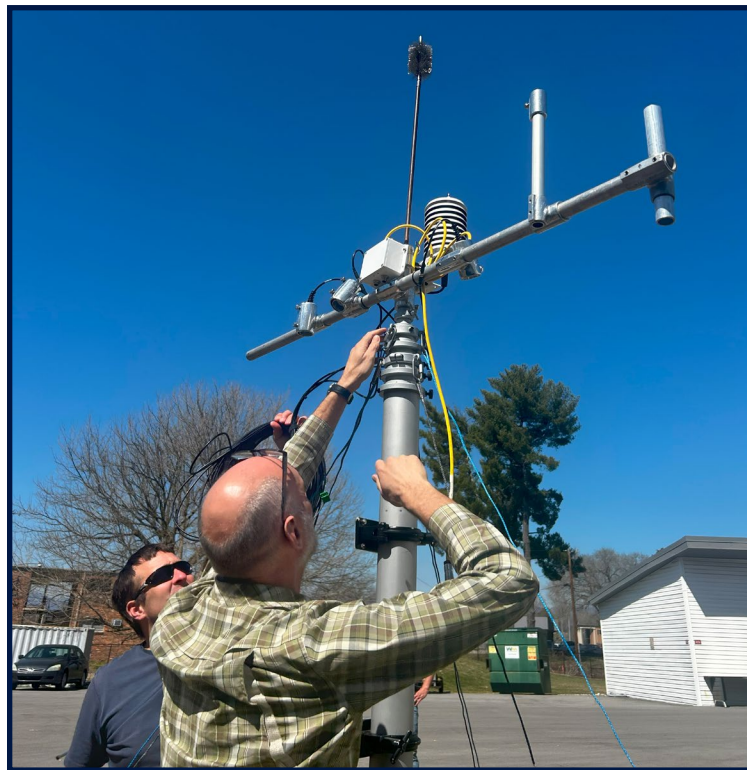
ATDD Director John Kochendorfer (left side in photo on left) and Physical Scientist Temple Lee (right side in left photo) test out set up of the rapid-deploy tower using instructions developed for easy set up by any experienced field scientist. Credit: Erica Massengill (NOAA/ORAU)
