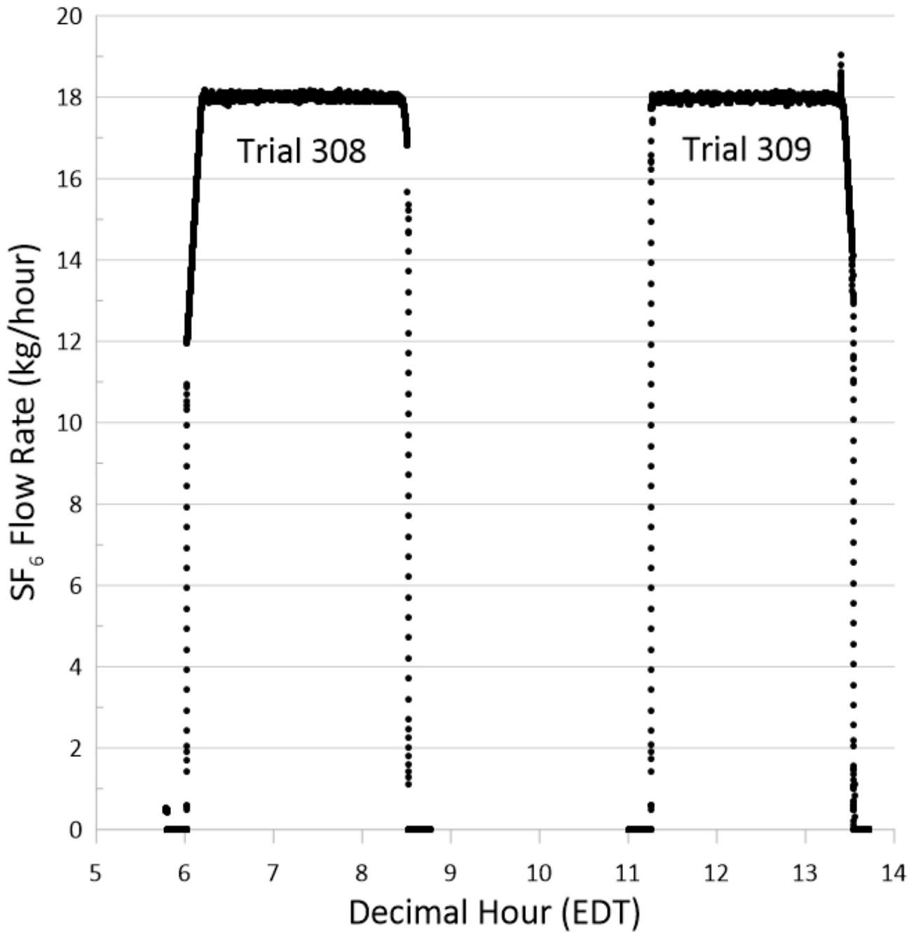
Figure 1. SF<sub>6</sub> flow rates from the blimp platform. Excursions in the release rate at release startup and end are inconsequential.
