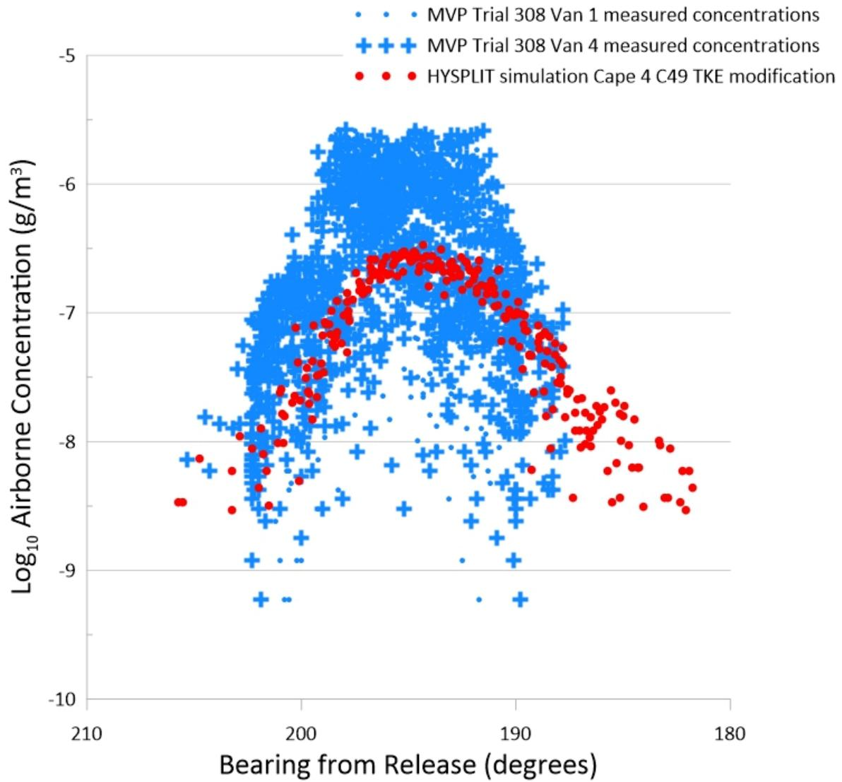
Figure 22 Trial 308 predicted and observed airborne concentration levels between 18.75 and 19.25 km downwind of the tracer release point using the C49 WRF TKE simulation
