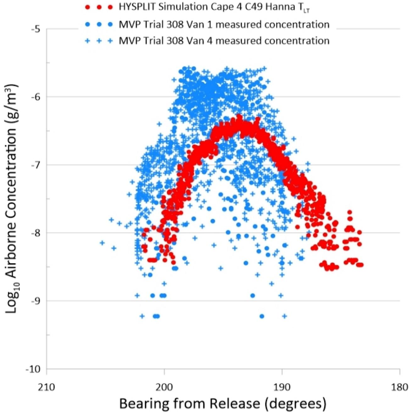
Figure 23 Trial 308 predicted and observed airborne concentration levels between 18.75 and 19.25 km downwind of the tracer release point using the C49 WRF Hanna T<sub>LT</sub> simulation.
