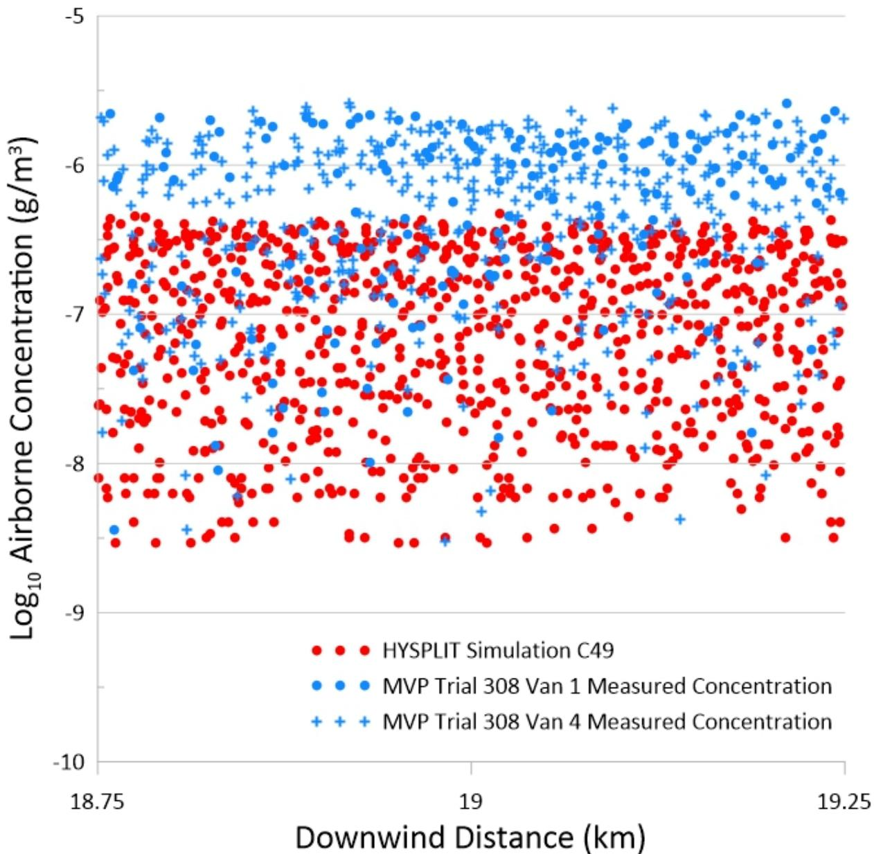
Figure 18 Trial 308 predicted and observed airborne concentration levels between 18.75 and 19.25 km downwind of the tracer release point using the C49 WRF simulation.
