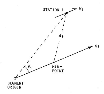
Figure 2. Configuration for determining the contribution  $S_i$  in a trajectory segment calculation from average wind  $W_i$  at station i.
