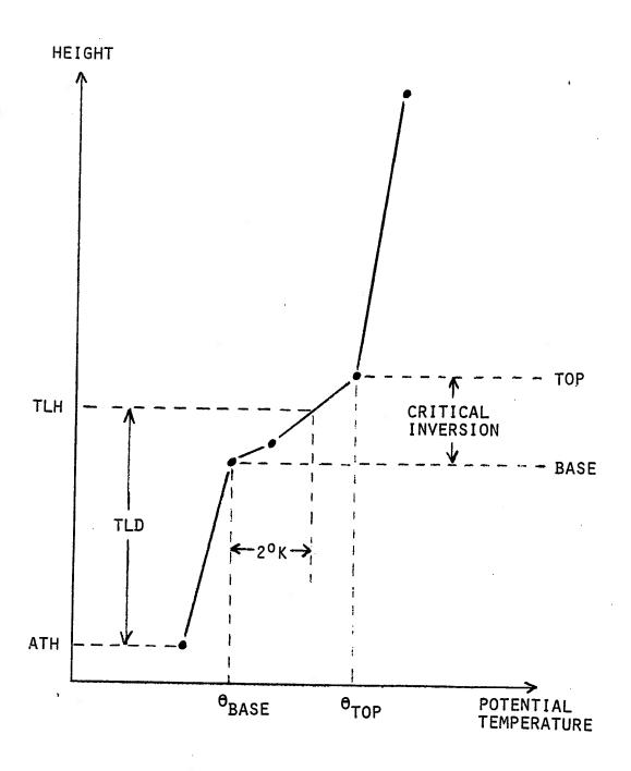
Figure 1. Schematic diagram for determining the transport layer depth (TLD). TLH refers to the transport layer height and ATH to the average terrain height.
