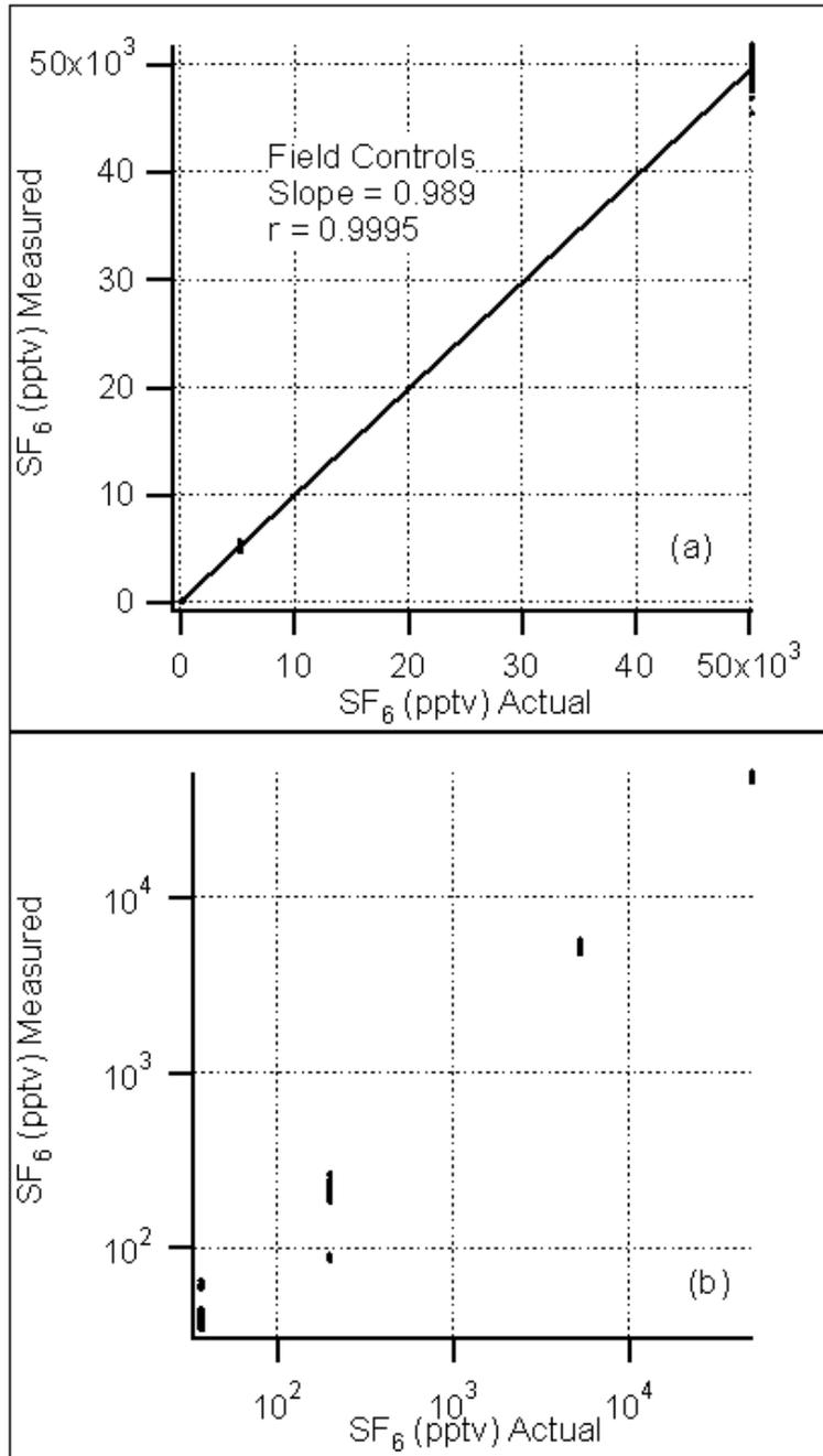
Figure 39. Plots of field control samples expressed (a) linearly with linear regression results and (b) logarithmically to better illustrate the low end results. The lone Test 2 outlier for the 199.5 pptv standard is apparent.
