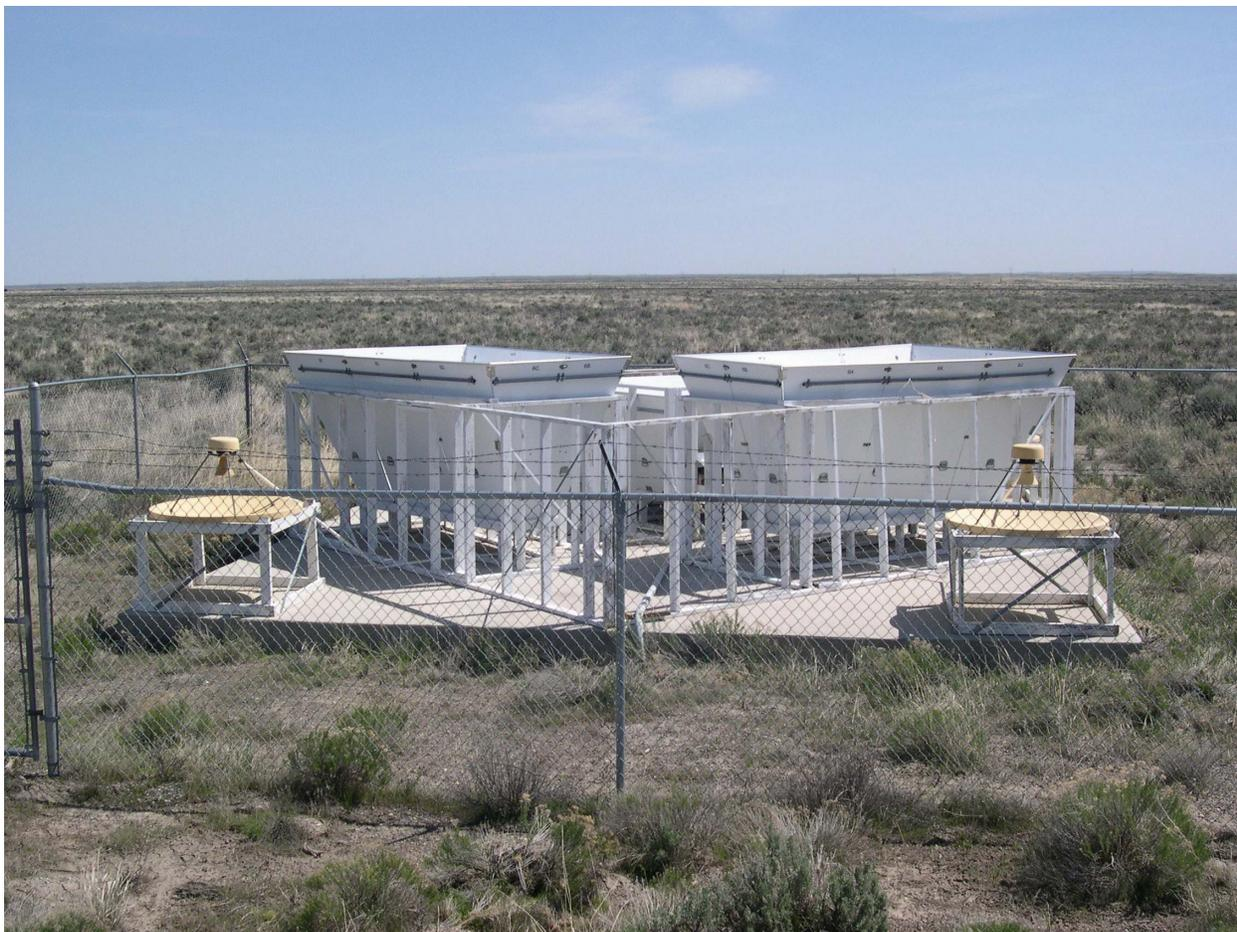
Figure 66. Radar wind profiler and RASS measured the upper wind and temperature profiles during RSBTS08.
