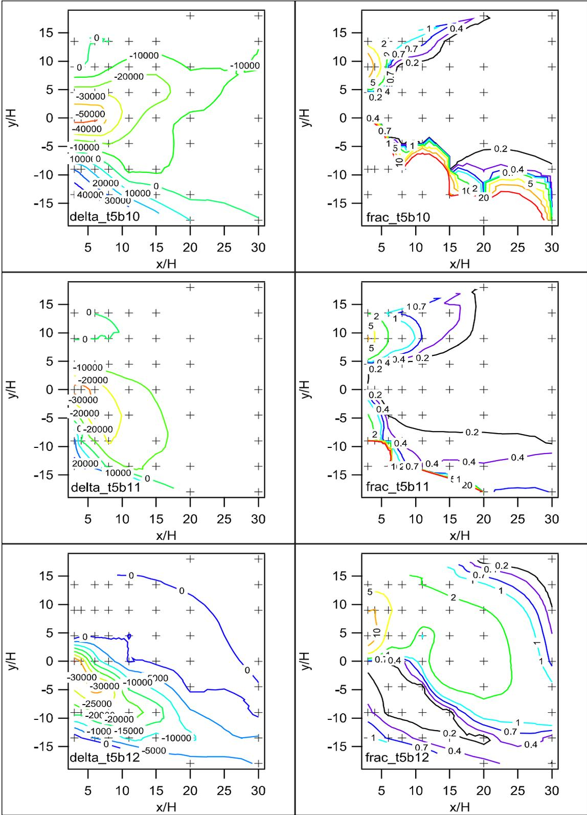
Figure 136. Comparison between barrier and non-barrier grids for difference (delta) and ratio (frac) of concentrations at corresponding grid locations, Test 5, bags 10-12.
