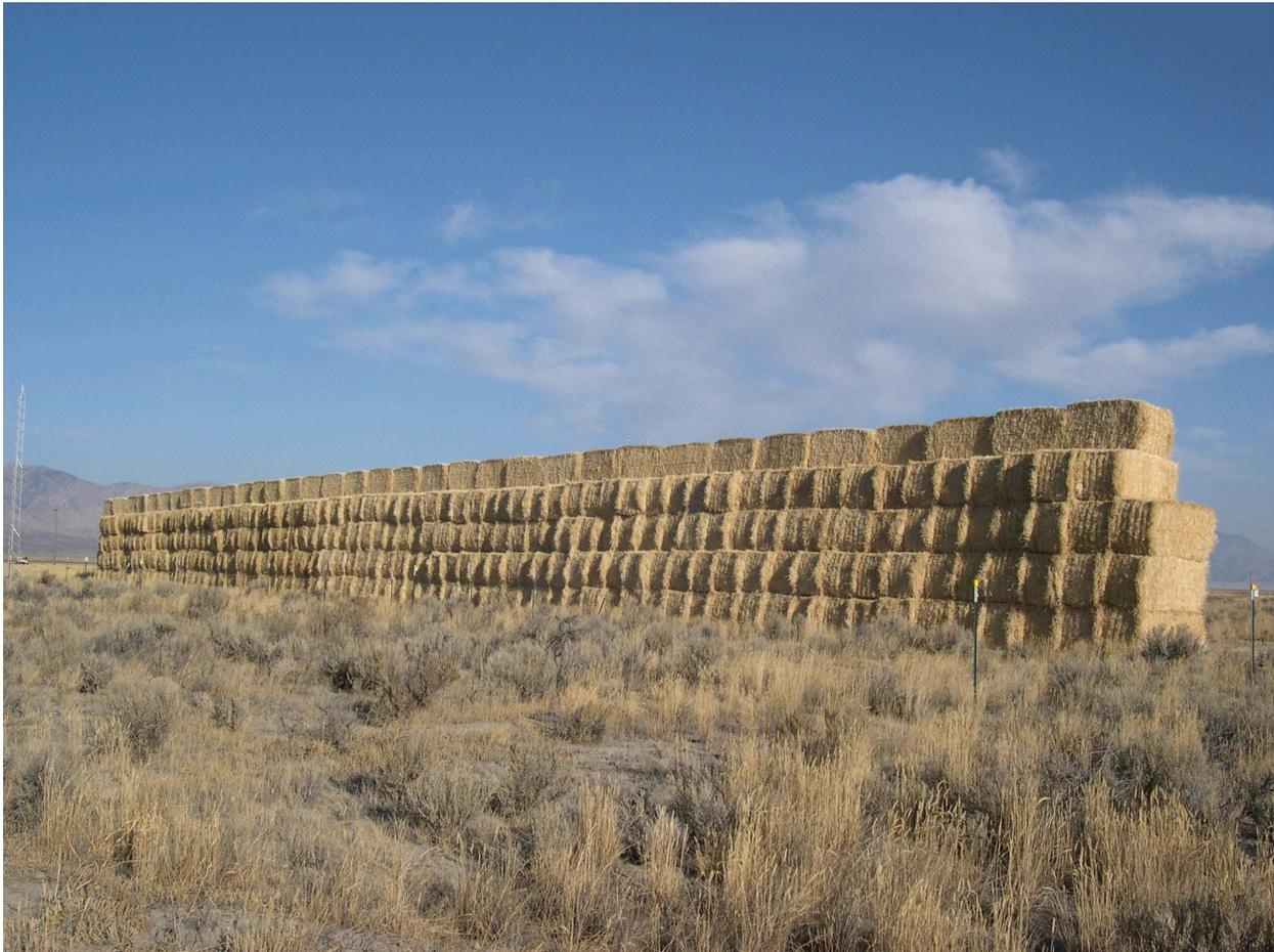
Figure 7. The mock sound barrier was constructed of 300 1-ton straw bales and was 6 m in height and 90 m in length.
