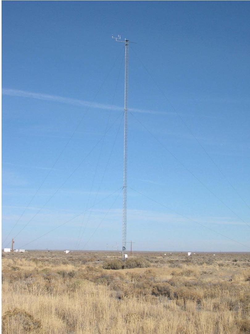
Figure 62. Command center meteorological tower monitored the current winds during the project.
