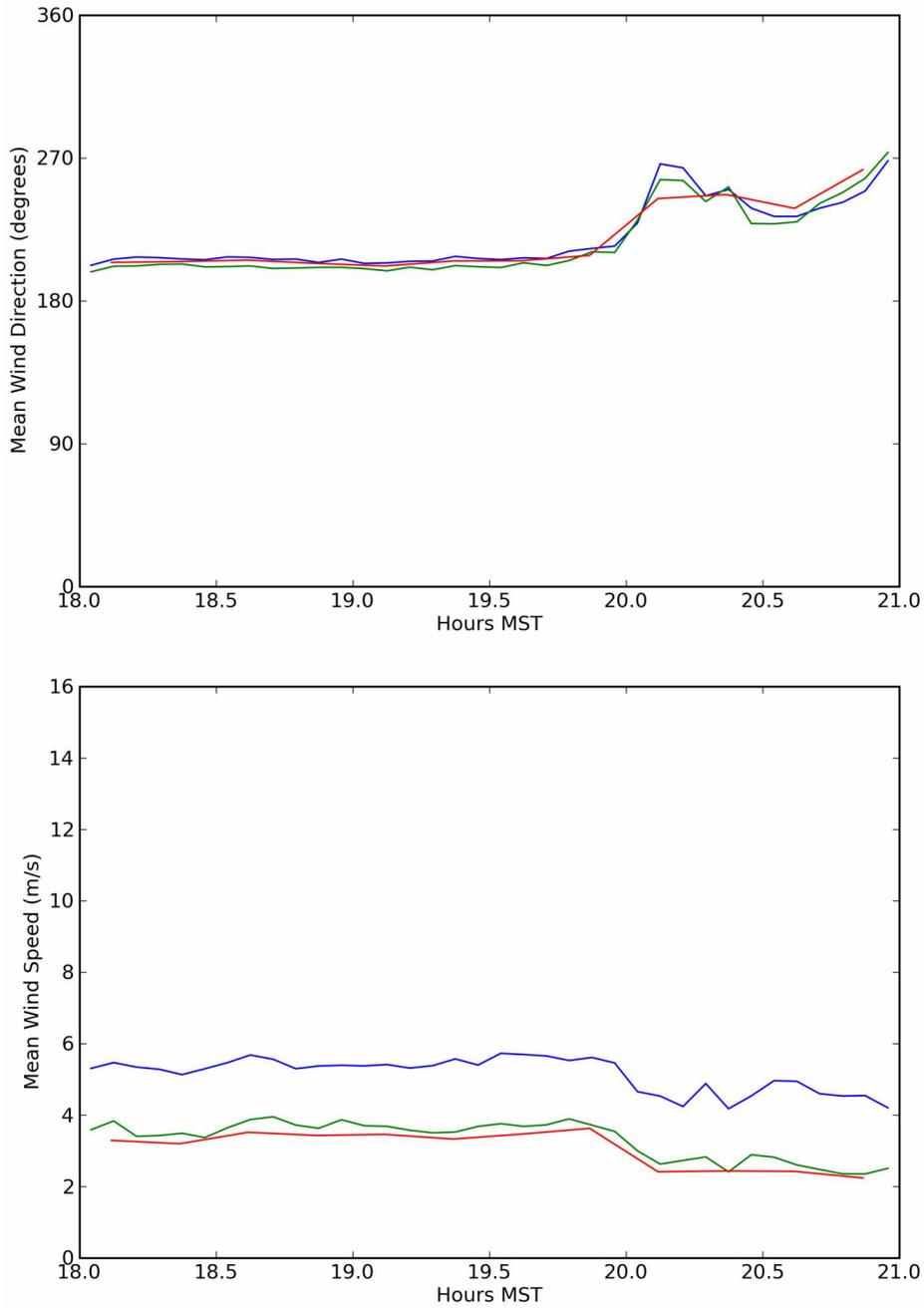
Figure 69. Wind speed and direction plots for the non-barrier sonic (R5) (red), 3 m command center meteorological tower (green), and 10 m GRI tower (blue) during Test 3.
