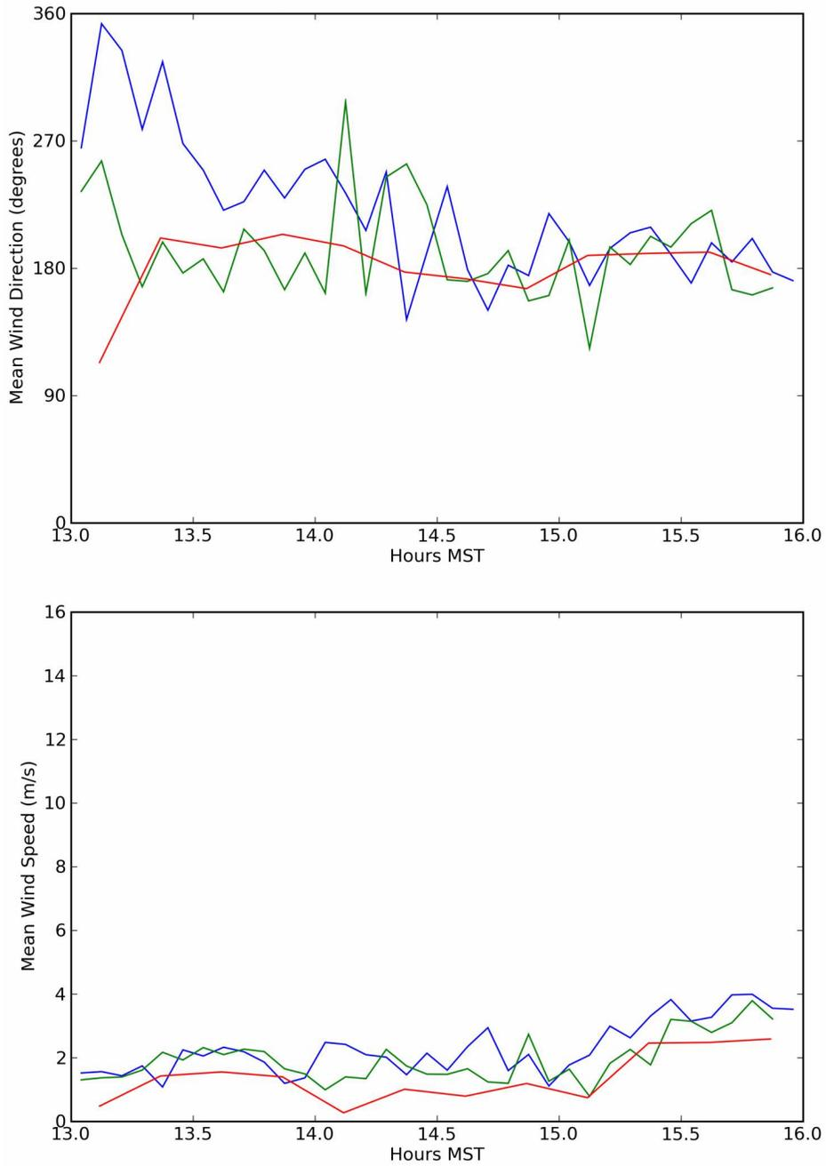
Figure 68. Wind speed and direction plots for the non-barrier sonic (R5) (red), 3 m command center meteorological tower (green), and 10 m GRI tower (blue) during Test 2.
