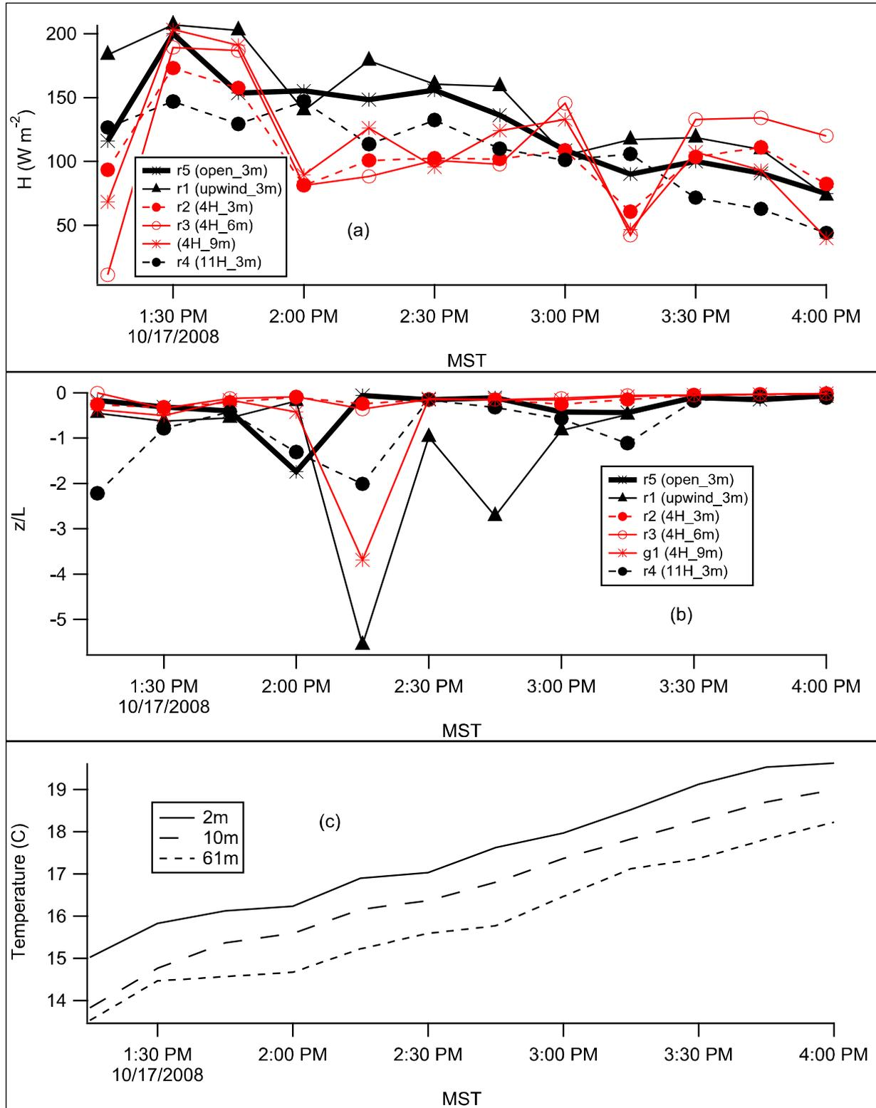
Figure 92. Test 2 sonic anemometer results for (a) sensible heat flux  $H$ , (b) stability parameter  $z/L$ , and (c) vertical temperature gradient at the Grid 3 tower.
