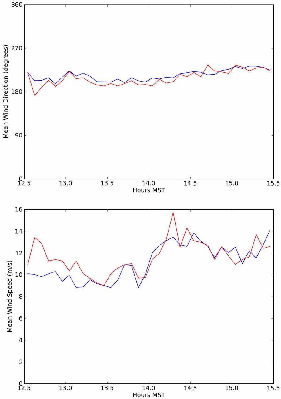
Figure 72. Wind speed and direction comparison plots of the 60 m sodar level (red) and the 60 m GRI Mesonet tower (blue) for Test 1.
