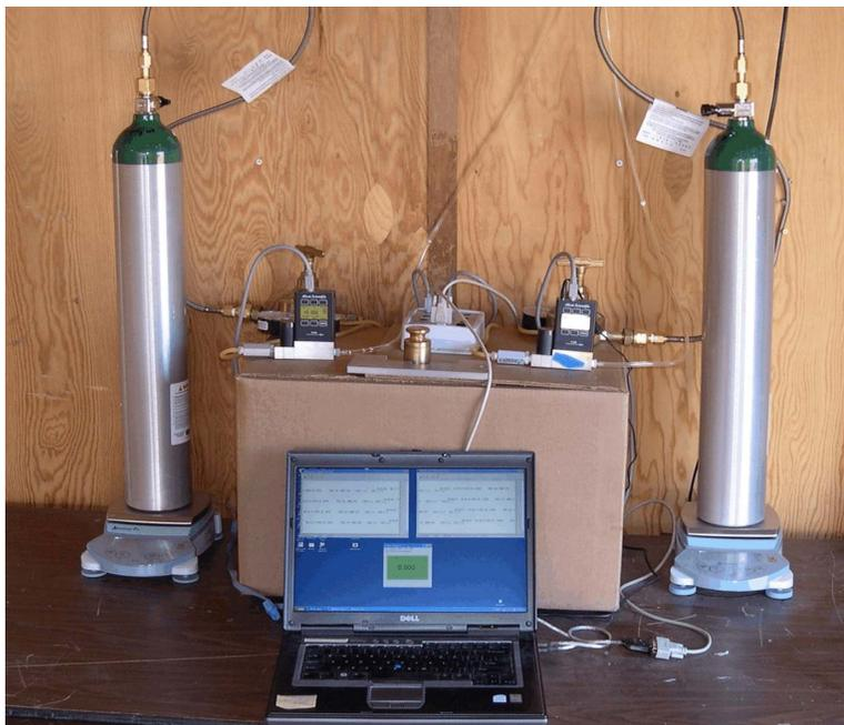
Figure 8. The SF<sub>6</sub> release system inside the cargo trailer including the SF<sub>6</sub> bottles, mass flow controllers, computer data acquisition and control system, and electronic scales under the bottles.
