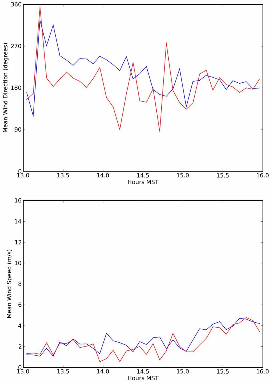
Figure 73. Wind speed and direction comparison plots of the 60 m sodar level (red) and the 60 m GRI Mesonet tower (blue) for Test 2.
