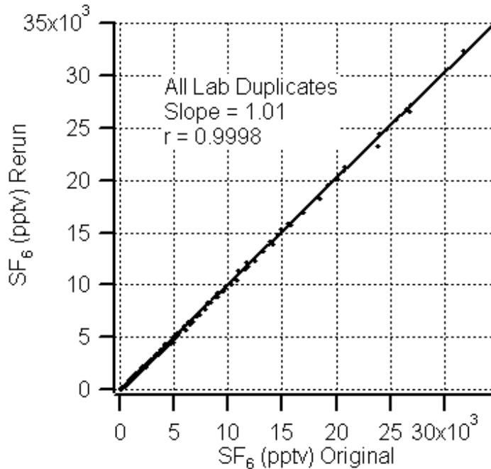
Figure 38. Linear regression of rerun against original values for all laboratory duplicates.
