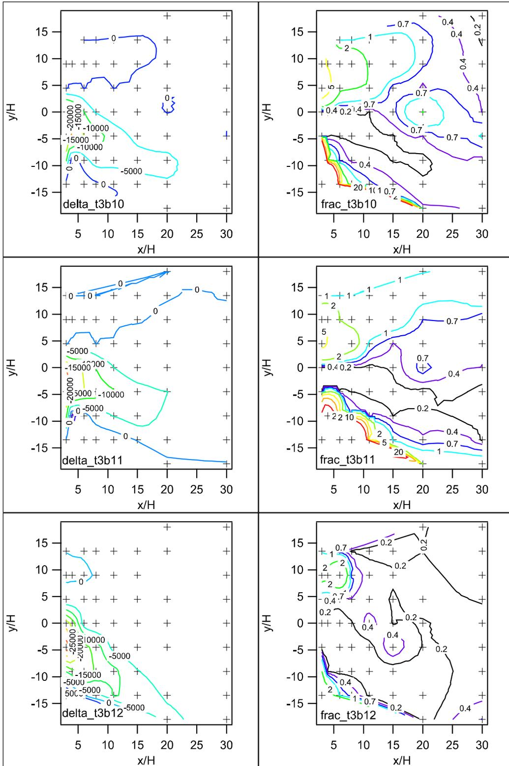
Figure 114. Comparison between barrier and non-barrier grids for difference ( $\Delta$ ) and ratio ( $\text{frac}$ ) of concentrations at corresponding grid locations, Test 3, bags 10-12.
