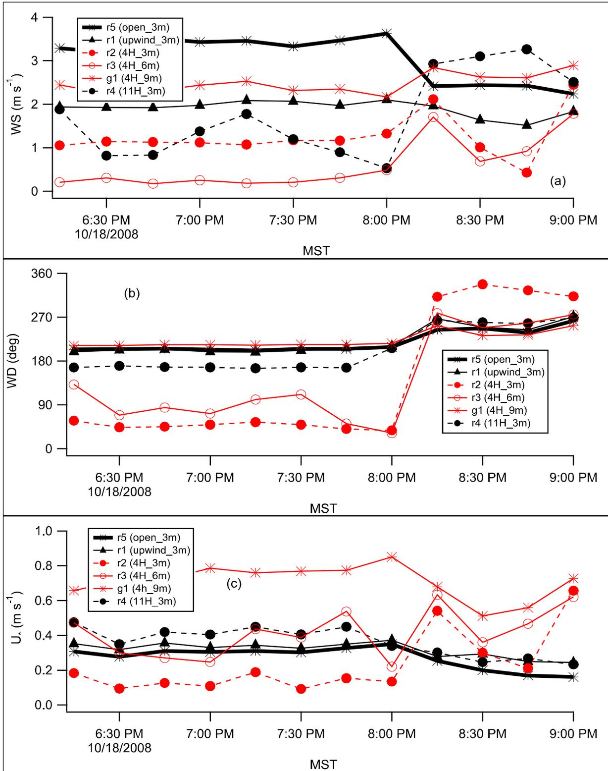
Figure 105. Test 3 sonic anemometer results for (a) wind speed, (b) wind direction, and (c) friction velocity  $u_*$ .
