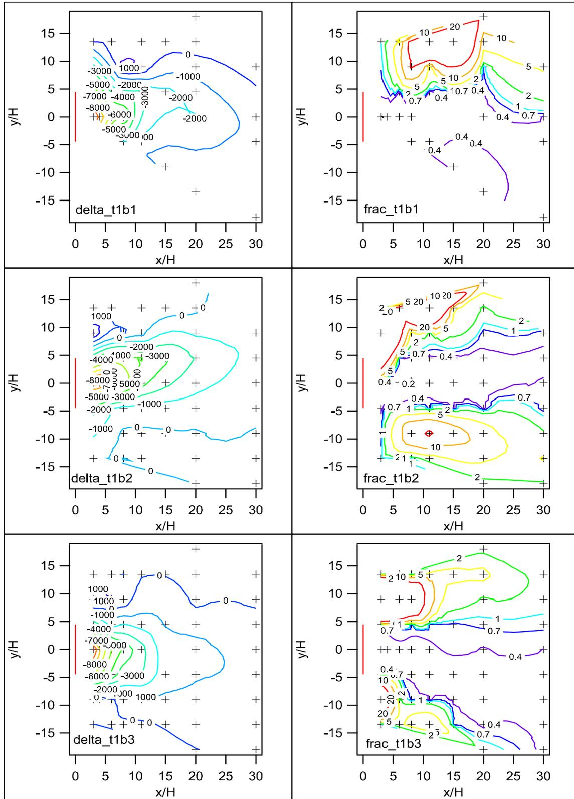
Figure 83. Comparison between barrier and non-barrier grids for difference (delta) and ratio (frac) of concentrations at corresponding grid locations, Test 1, bags 1-3.
