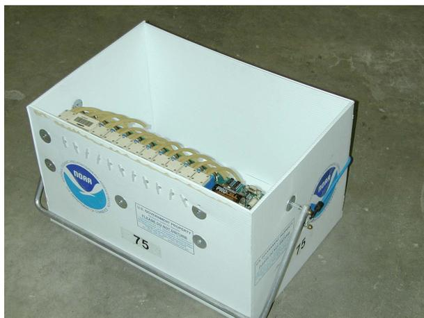
Figure 21. Bag sampler with cover and cartridge removed.
