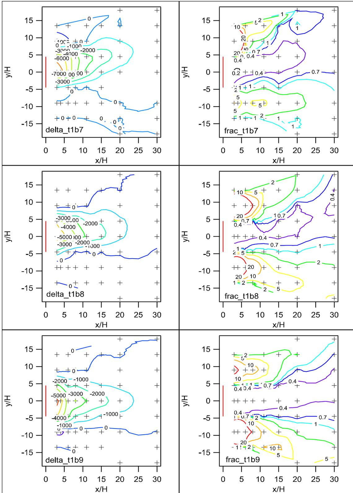
Figure 85. Comparison between barrier and non-barrier grids for difference (delta) and ratio (frac) of concentrations at corresponding grid locations, Test 1, bags 7-9.
