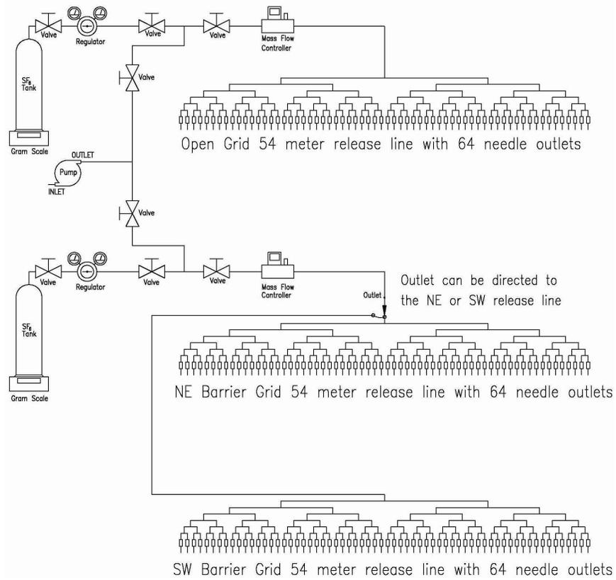
Figure 10. Diagram of the SF<sub>6</sub> release system for the open grid and either side of the barrier grid area.
