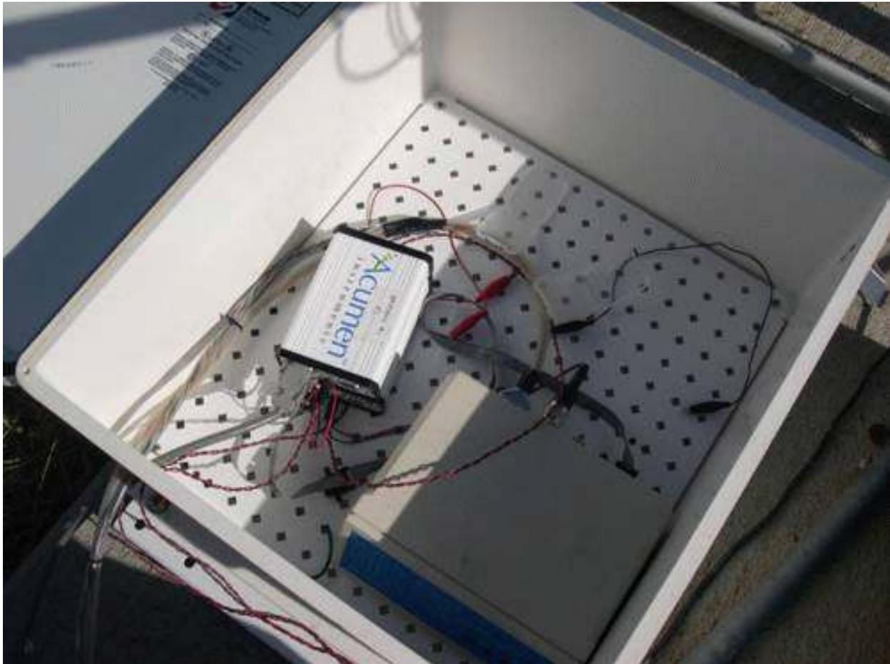
Figure 58. An Acumen data collection bridge (white device inside box) is used to collect data from the sonic anemometers.
