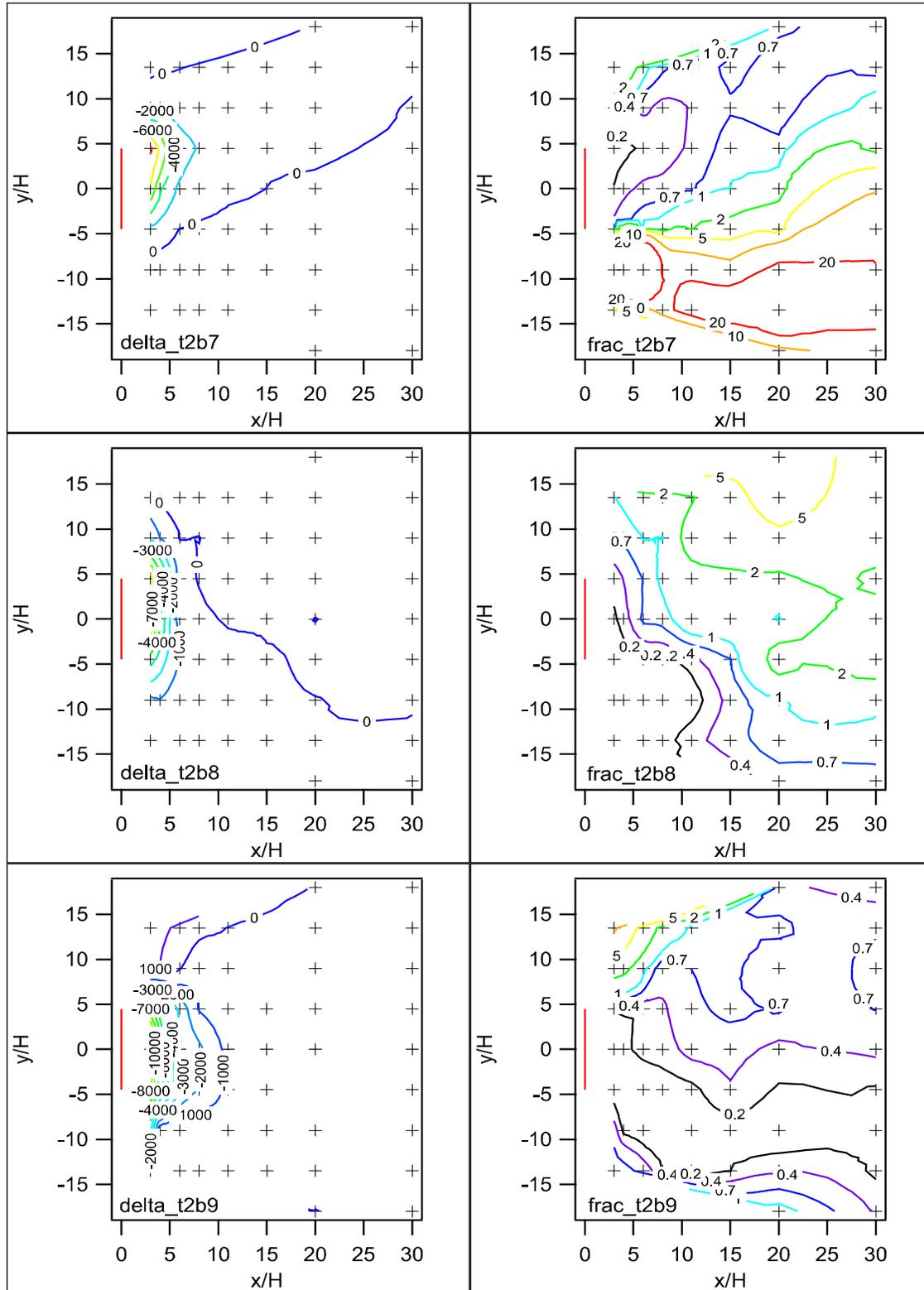
Figure 99. Comparison between barrier and non-barrier grids for difference (delta) and ratio (frac) of concentrations at corresponding grid locations, Test 2, bags 7-9.
