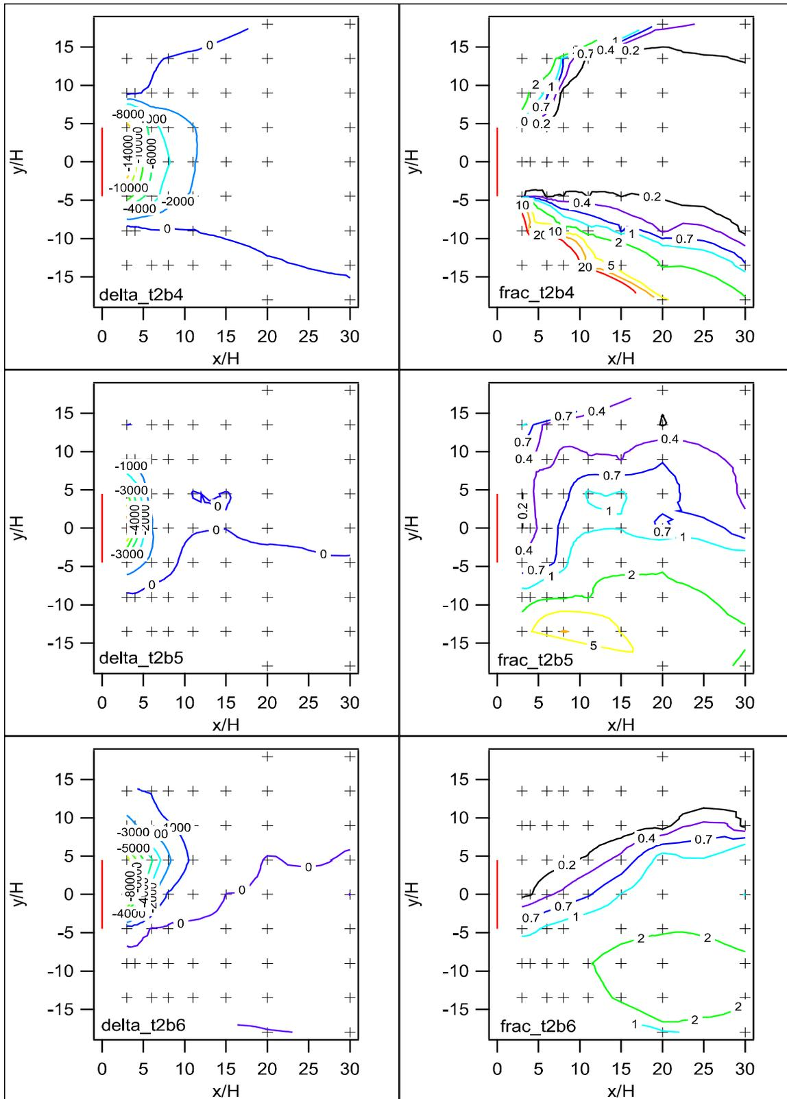
Figure 98. Comparison between barrier and non-barrier grids for difference (delta) and ratio (frac) of concentrations at corresponding grid locations, Test 2, bags 4-6.
