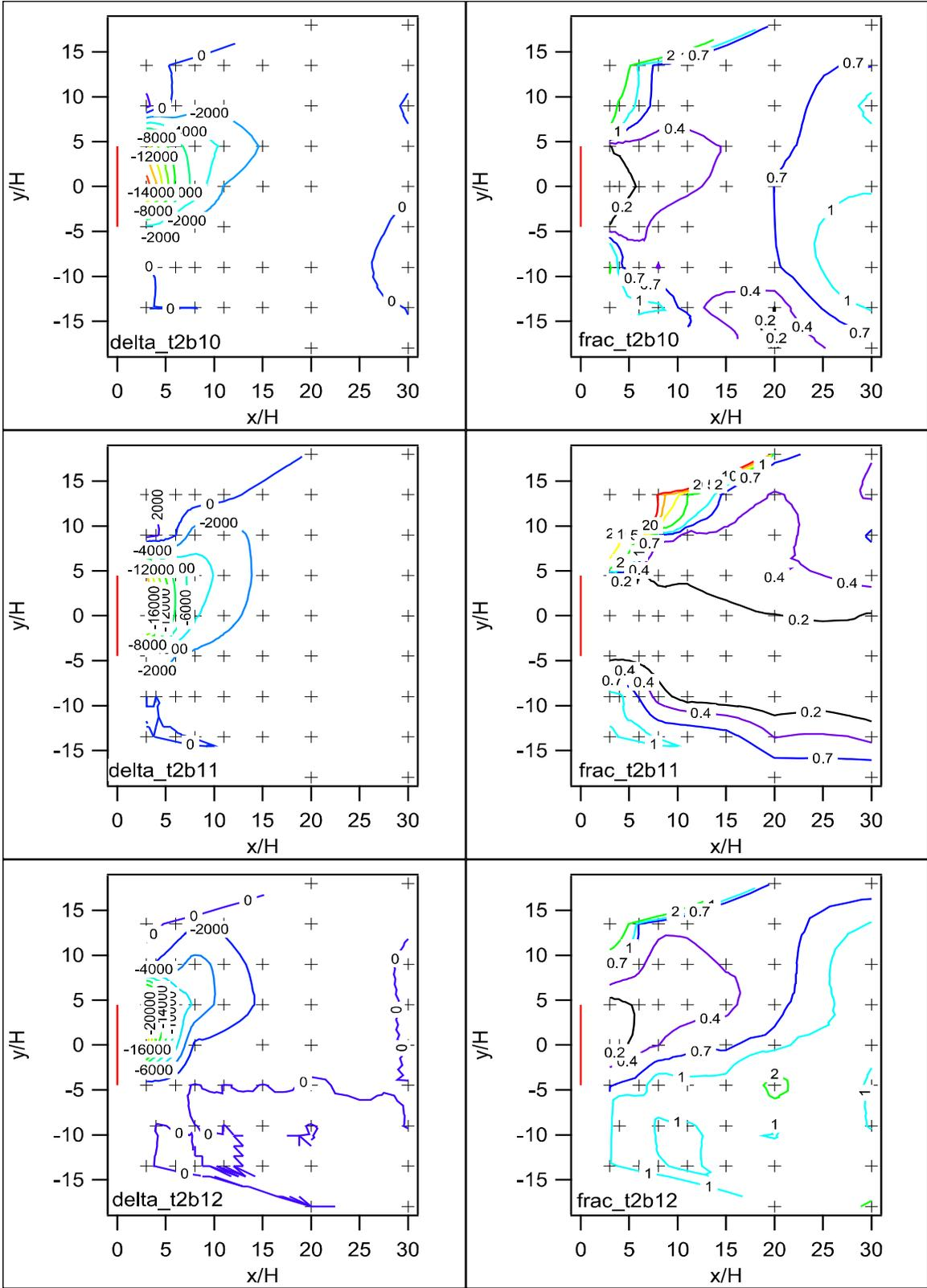
Figure 100. Comparison between barrier and non-barrier grids for difference (delta) and ratio (frac) of concentrations at corresponding grid locations, Test 2, bags 10-12.
