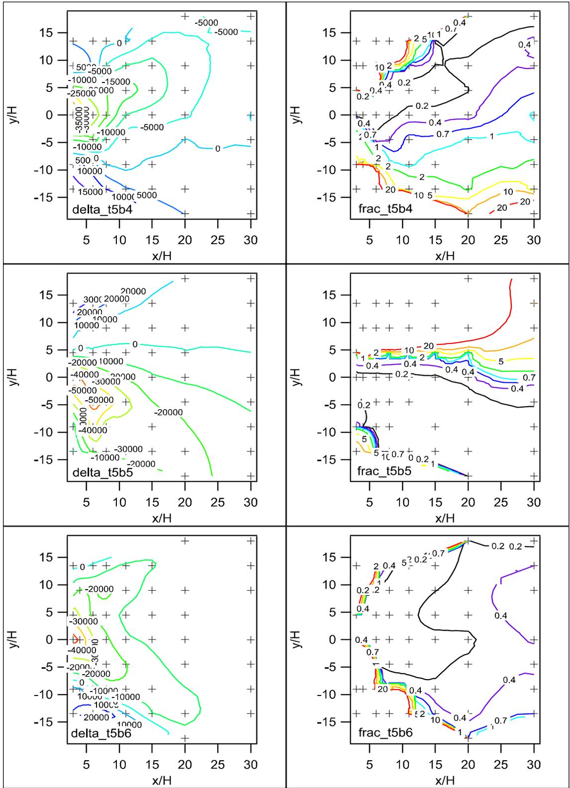
Figure 134. Comparison between barrier and non-barrier grids for difference ( $\Delta$ ) and ratio ( $\text{frac}$ ) of concentrations at corresponding grid locations, Test 5, bags 4-6.
