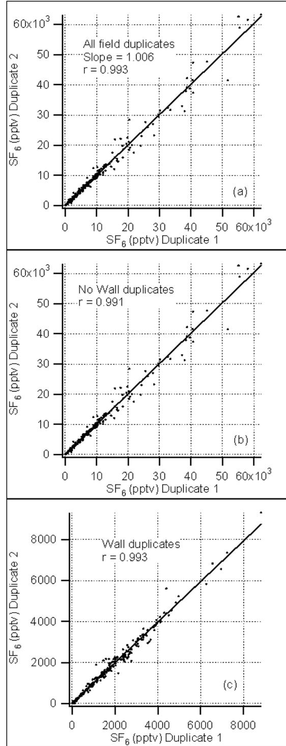
Figure 40. Linear regressions for (a) all field duplicate samples combined, (b) non-barrier duplicate samples only, and (c) barrier duplicate samples only.
