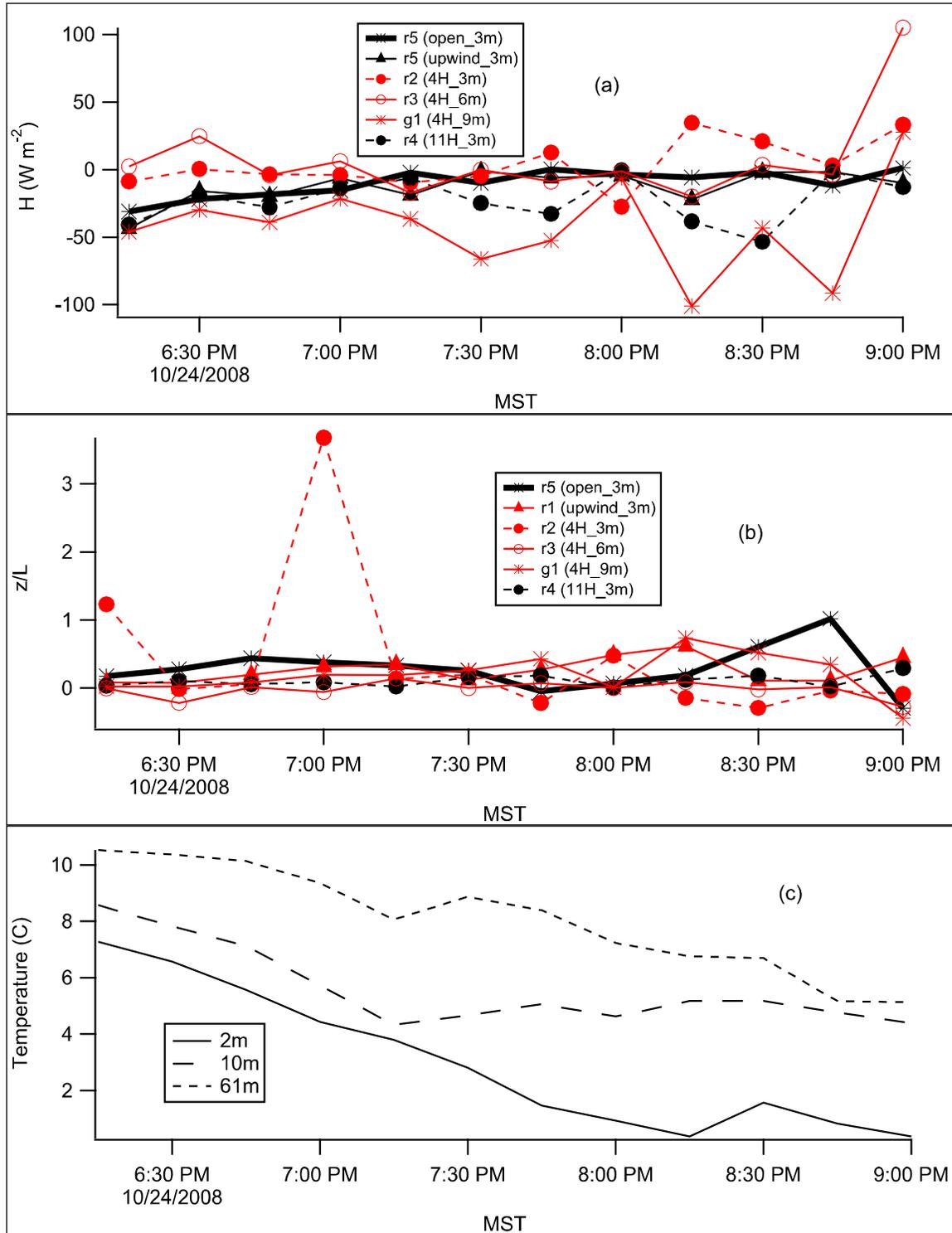
Figure 128. Test 5 sonic anemometer results for (a) sensible heat flux  $H$ , (b) stability parameter  $z/L$ , and (c) vertical temperature gradient at the Grid 3 tower.
