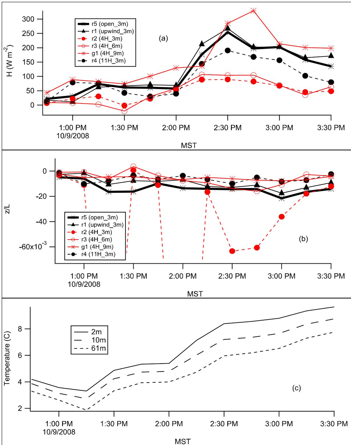
Figure 78. Test 1 sonic anemometer results for (a) sensible heat flux  $H$ , (b) stability parameter  $z/L$ , and (c) vertical temperature gradient at the Grid 3 tower.
