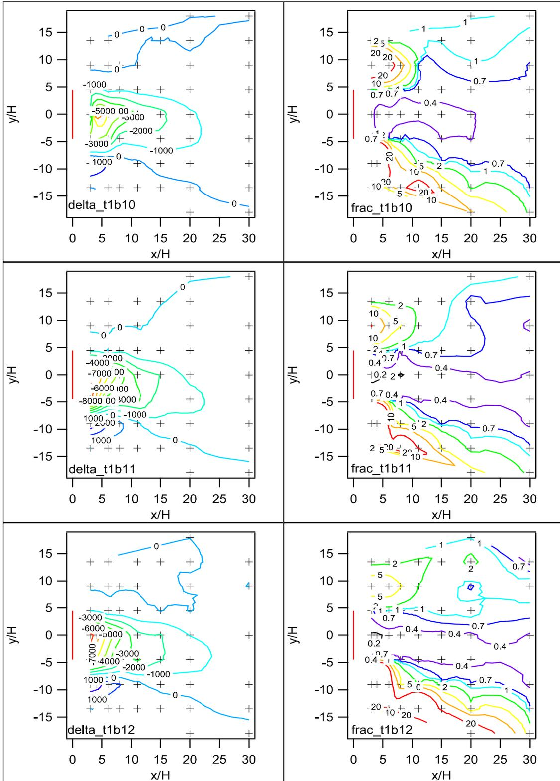
Figure 86. Comparison between barrier and non-barrier grids for difference (delta) and ratio (frac) of concentrations at corresponding grid locations, Test 1, bags 10-12.
