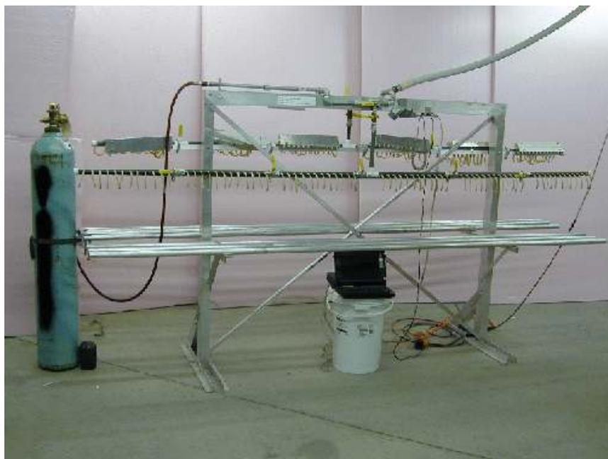
Figure 35. Cartridge cleaning apparatus.
