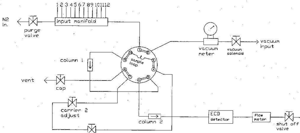
Figure 27. Schematic of injection to column 1 (pre-column) and on to column 2 (main column).
