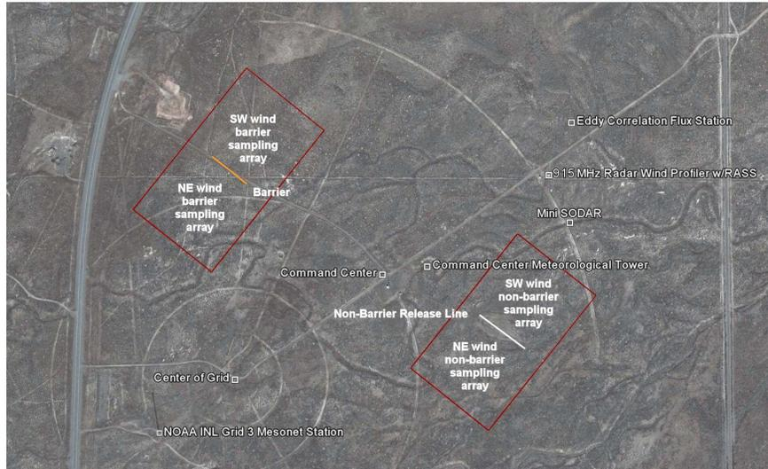
Figure 4. Diagram of the experimental set up at the Grid 3 area.
