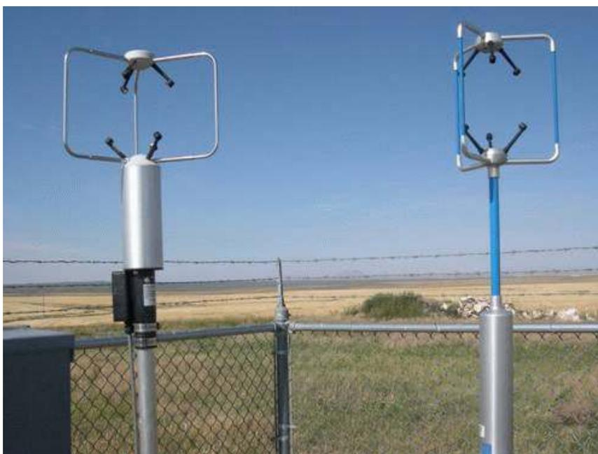
Figure 56. The two types of 3-D sonic anemometers deployed were a R. M. Young Ultrasonic 81000 (left) and a Gill Windmaster Pro (right).
