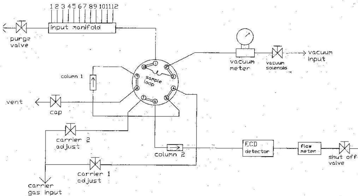
Figure 28. Schematic of sample loop fill with column 1 (pre-column) in the back-flush position.
