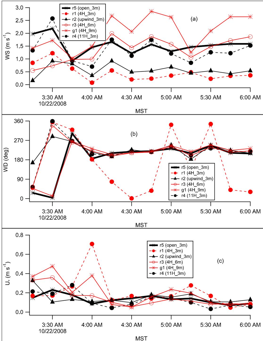
Figure 119. Test 4 sonic anemometer results for (a) wind speed, (b) wind direction, and (c) friction velocity  $u_*$ .
