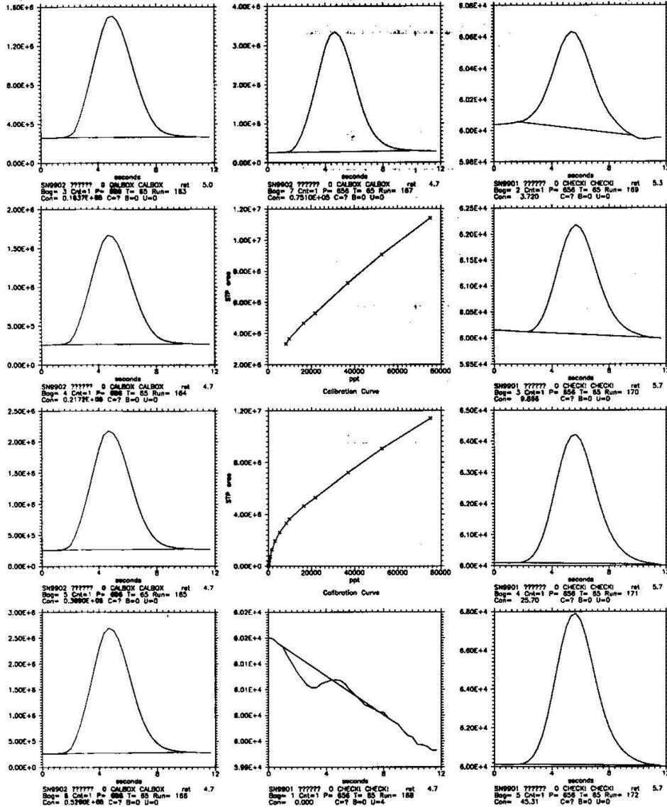
Figure 44. Example of chromatogram and calibration curve check sheet.
