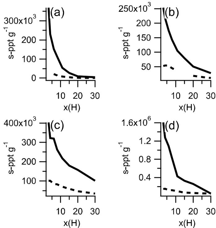
Figure 141. Comparison between non-barrier (solid) and barrier (dashed) normalized concentration profiles for (a) unstable, (b) neutral, c) weakly stable, and (d) stable cases.
