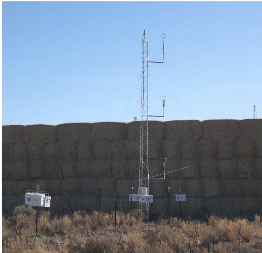
Figure 57. Vertical profile tower behind the barrier with the three anemometers at 3, 6, and 9 m. Also pictured are the programmable bag samplers hanging on the fence posts.
