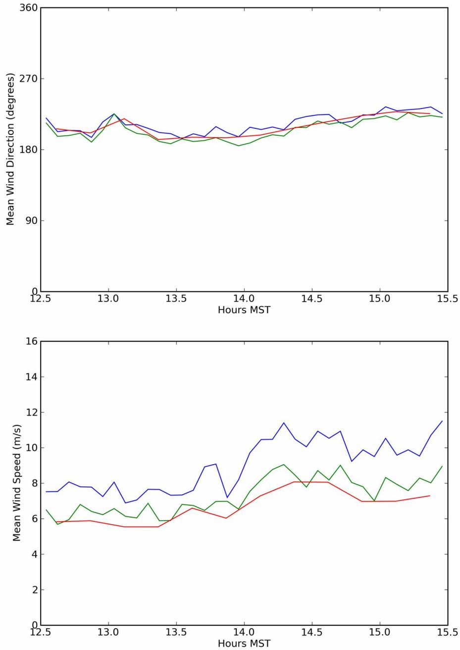
Figure 67. Wind speed and direction plots for the non-barrier sonic (R5) (red), 3 m command center meteorological tower (green), and 10 m GRI tower (blue) during Test 1.
