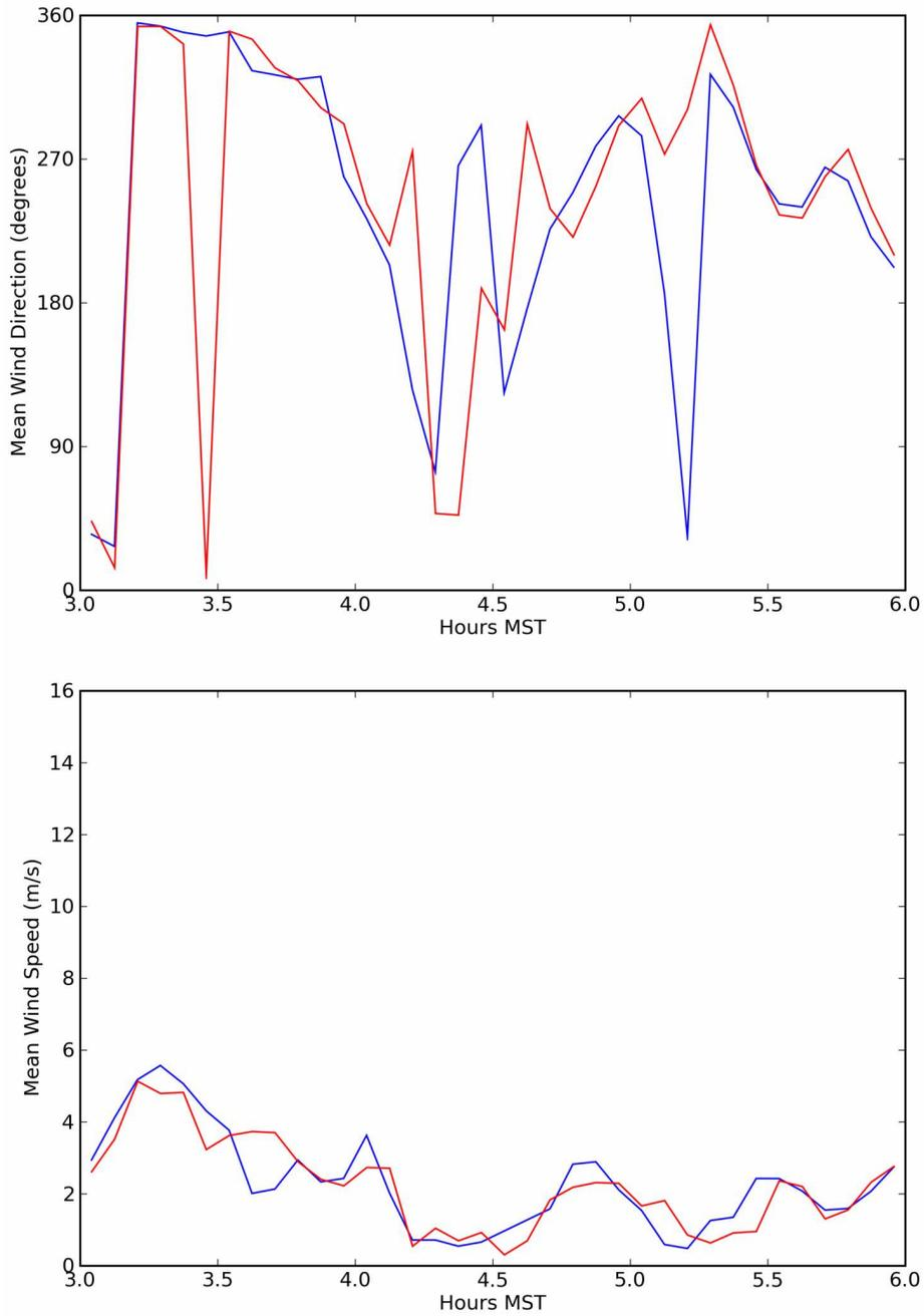
Figure 75. Wind speed and direction comparison plots of the 60 m sodar level (red) and the 60 m GRI Mesonet tower (blue) for Test 4.
