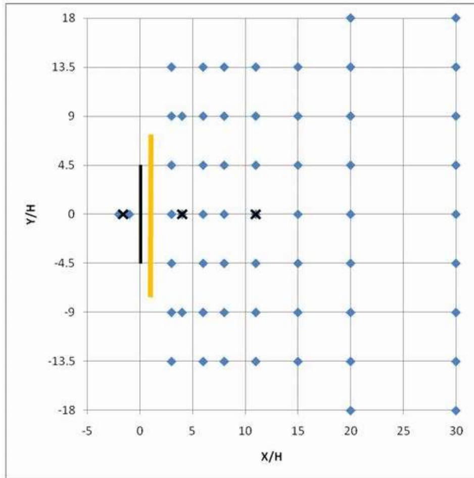
Figure 6. Schematic representation of the experimental plan showing the locations of the line source release on the left (bold), the barrier (orange), bag samplers (blue diamonds), and sonic anemometers (x). Sonic deployment heights at:  $X/H = -1.6$  ( $z = 3$  m on tower);  $X/H = 4$  ( $z = 3, 6,$  and  $9$  m on tower); and  $X/H = 11$  ( $z = 3$  m).  $H$  is the height of the barrier which was 6 m.
