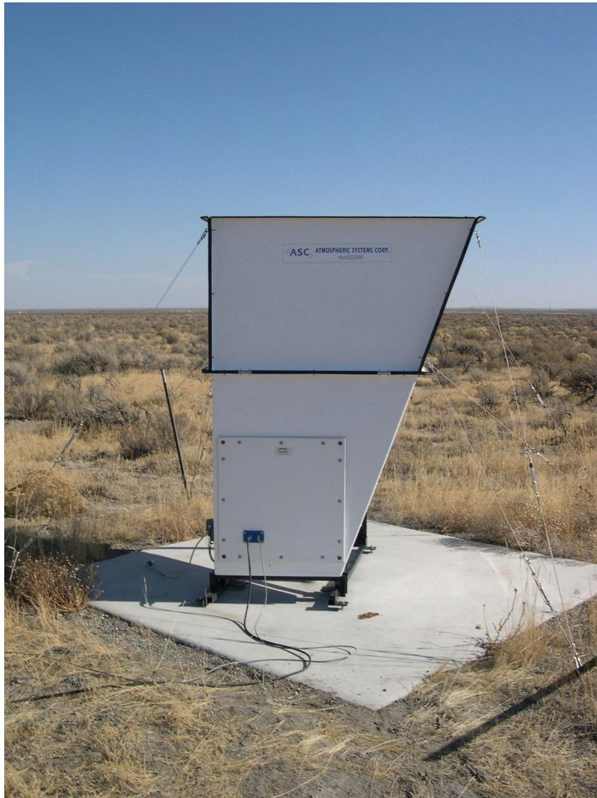
Figure 65. Mini sodar recorded vertical profiles of the wind speed and direction.
