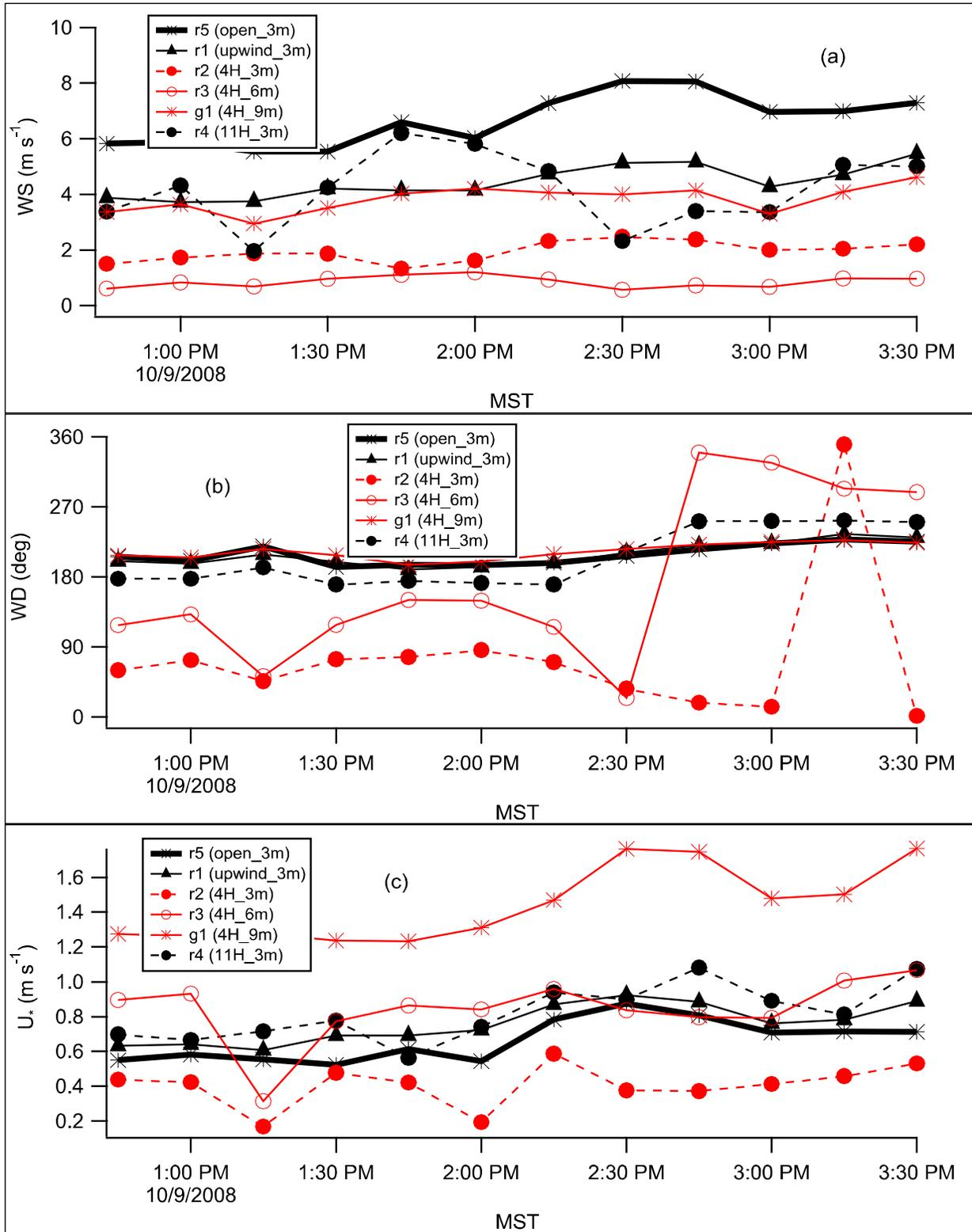
Figure 77. Test 1 sonic anemometer results for (a) wind speed, (b) wind direction, and (c) friction velocity  $u_*$ .
