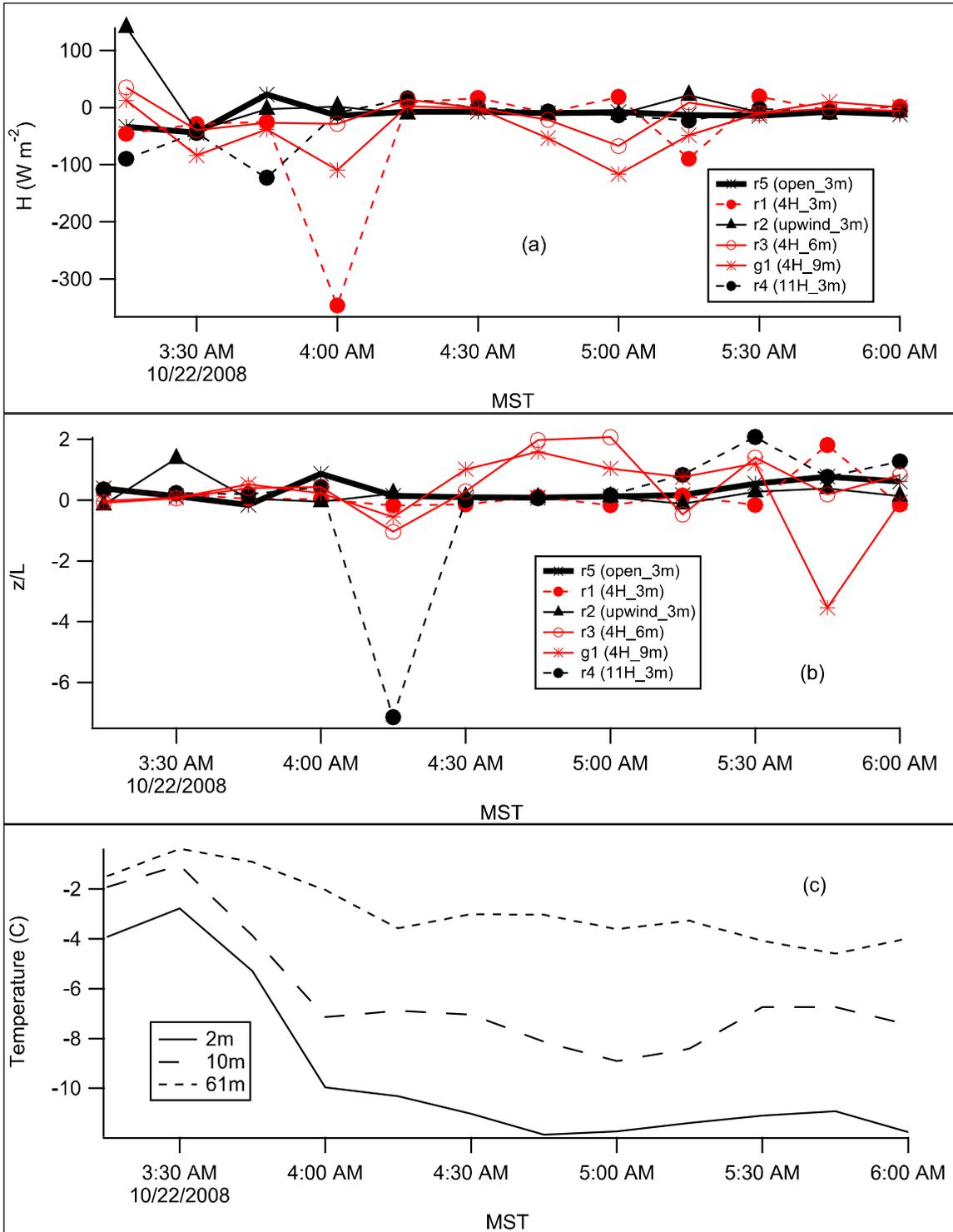
Figure 120. Test 4 sonic anemometer results for (a) sensible heat flux  $H$ , (b) stability parameter  $z/L$ , and (c) vertical temperature gradient at the Grid 3 tower.
