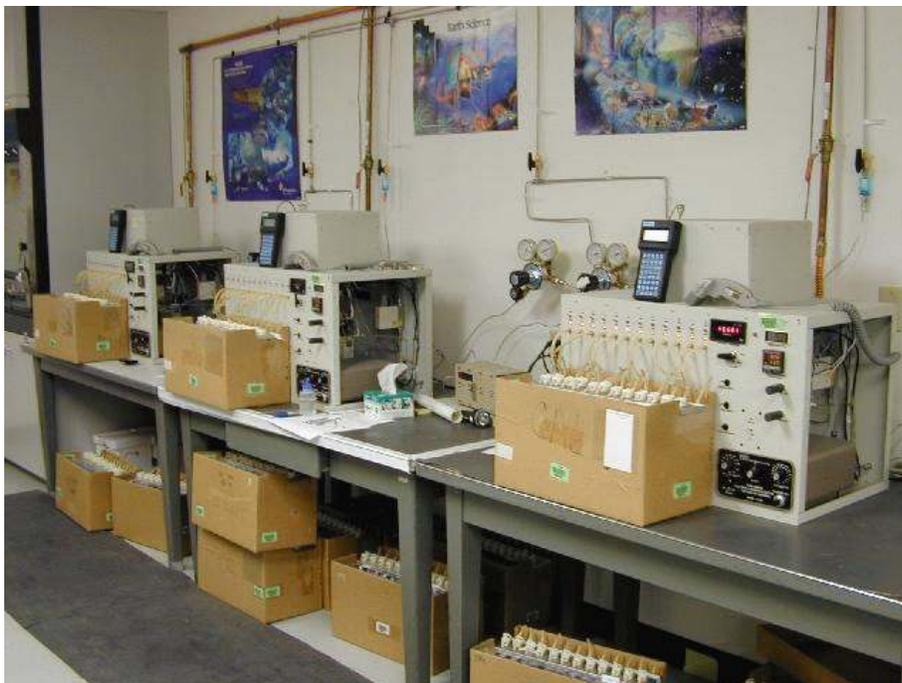
Figure 25. Three ATGASs attached to sample cartridges.
