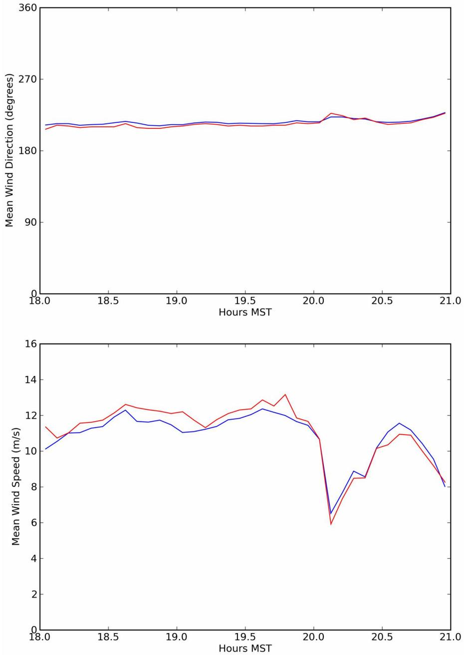
Figure 74. Wind speed and direction comparison plots of the 60 m sodar level (red) and the 60 m GRI Mesonet tower (blue) for Test 3.
