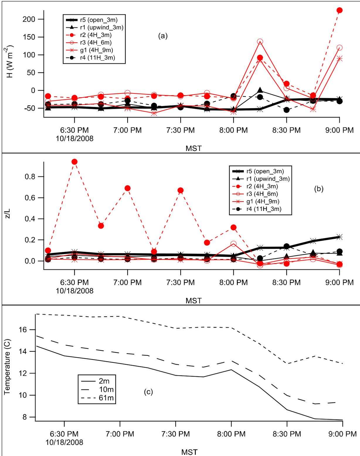
Figure 106. Test 3 sonic anemometer results for (a) sensible heat flux  $H$ , (b) stability parameter  $z/L$ , and (c) vertical temperature gradient at the Grid 3 tower.
