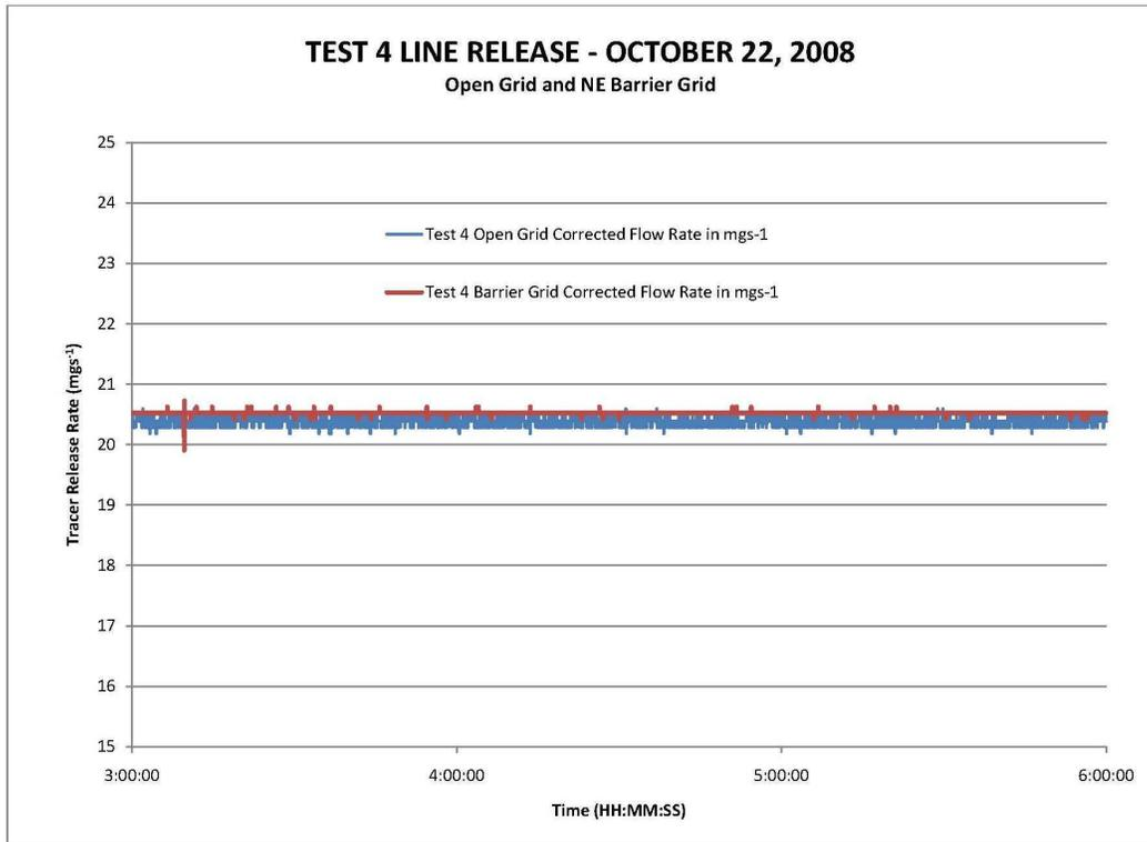
Figure 15. Tracer release rates for Test 4.
