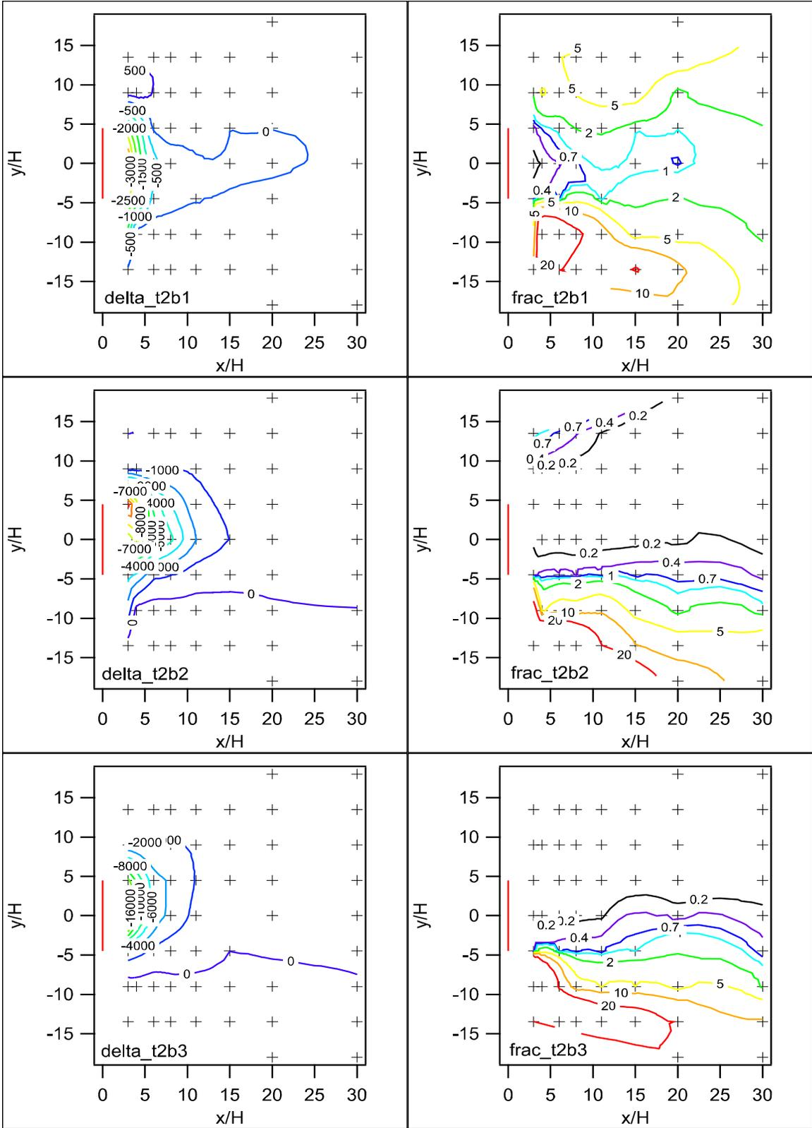
Figure 97. Comparison between barrier and non-barrier grids for difference (delta) and ratio (frac) of concentrations at corresponding grid locations, Test 2, bags 1-3.
