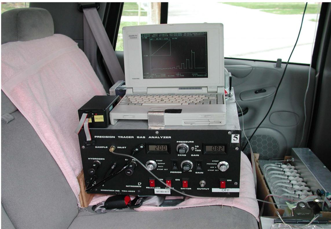
Figure 52. NOAA mobile tracer gas analyzer system, consisting of a laptop computer, a TGA-4000 below the laptop, and a calibration gas cartridge (lower right) installed in the rear seat of an SUV.
