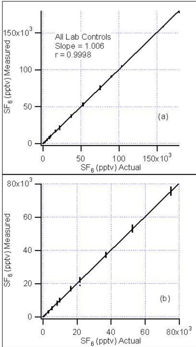
Figure 37. Comparison between measured and NIST-certified standard concentrations for (a) all lab control (CCV) samples and (b) CCV samples covering the concentration standards routinely used (3.49 to 75,100 pptv).
