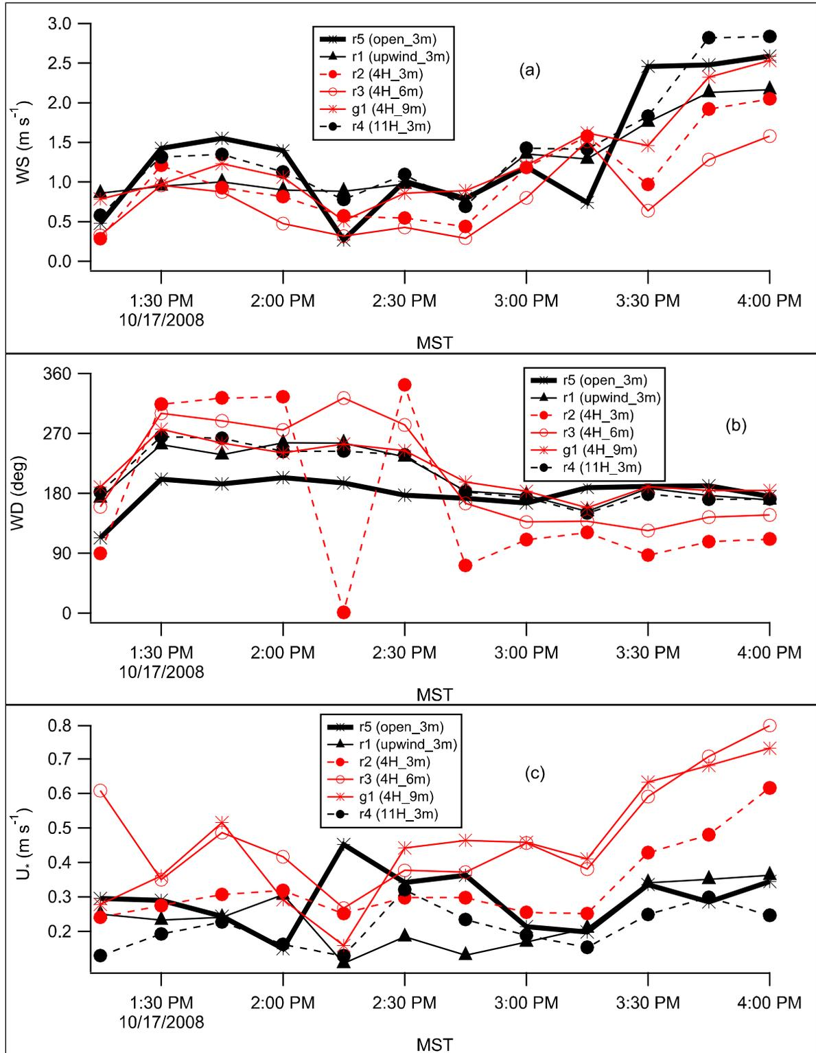
Figure 91. Test 2 sonic anemometer results for (a) wind speed, (b) wind direction, and (c) friction velocity  $u_*$ .
