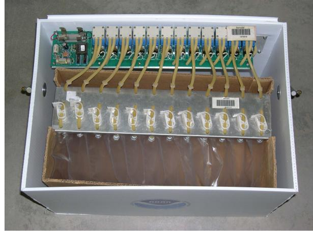
Figure 24. Bag sampler with sampler cartridge installed.
