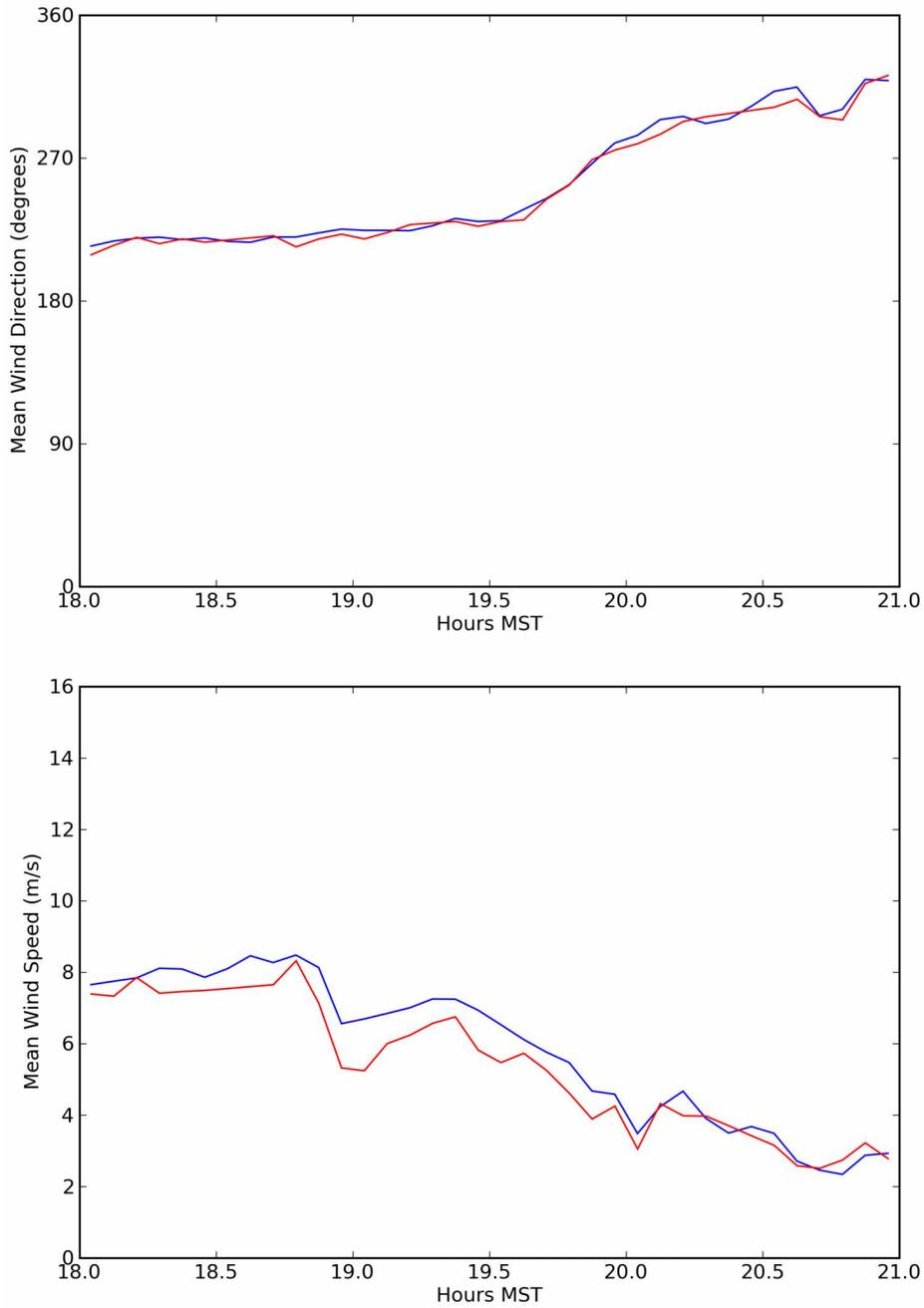
Figure 76. Wind speed and direction comparison plots of the 60 m sodar level (red) and the 60 m GRI Mesonet tower (blue) for Test 5.
