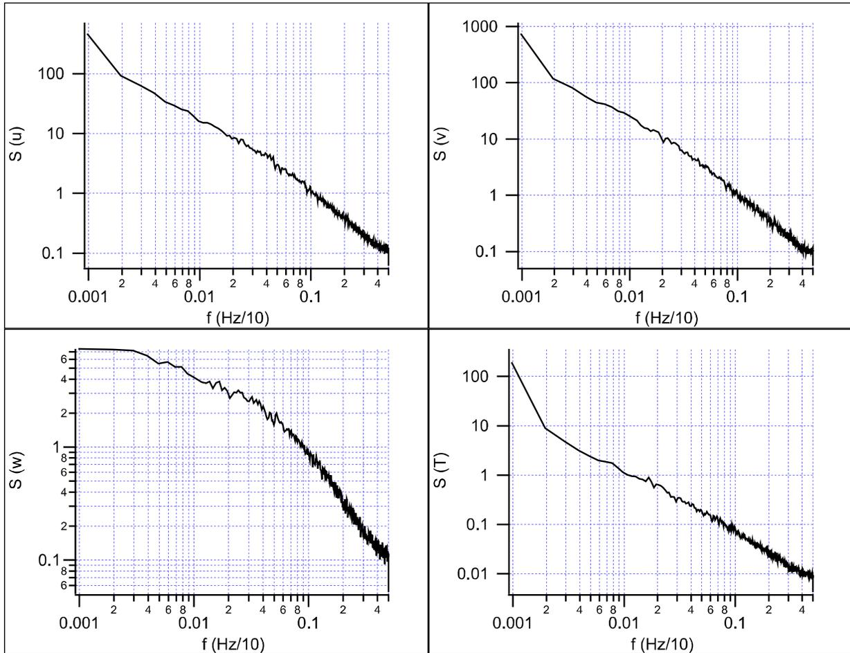
Figure 61. The spectra of u, v, w, and t for sonic R5 during Test 1.
