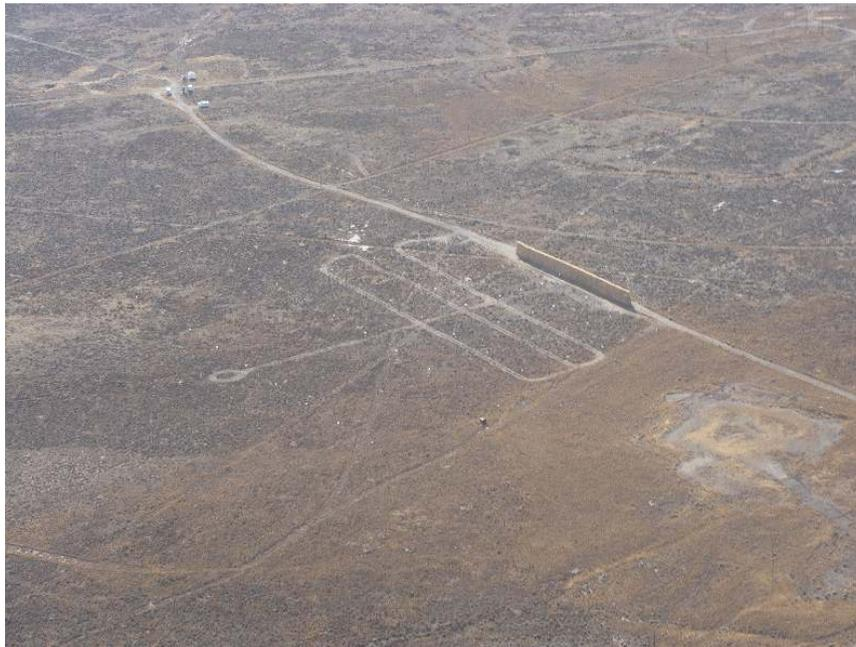
Figure 5. Aerial view of the barrier release area. The tracks on the near side of the barrier are the fast response analyzer route for SW winds. The release trailer and command center are visible in the upper left. The non-barrier release site is off the image to the upper left.
