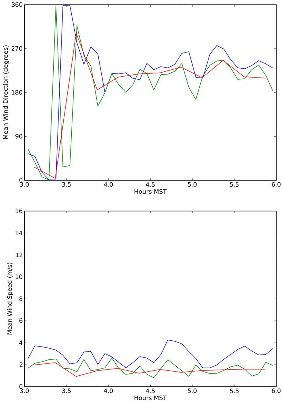
Figure 70. Wind speed and direction plots for the non-barrier sonic (R5) (red), 3 m command center meteorological tower (green), and 10 m GRI tower (blue) during Test 4.
