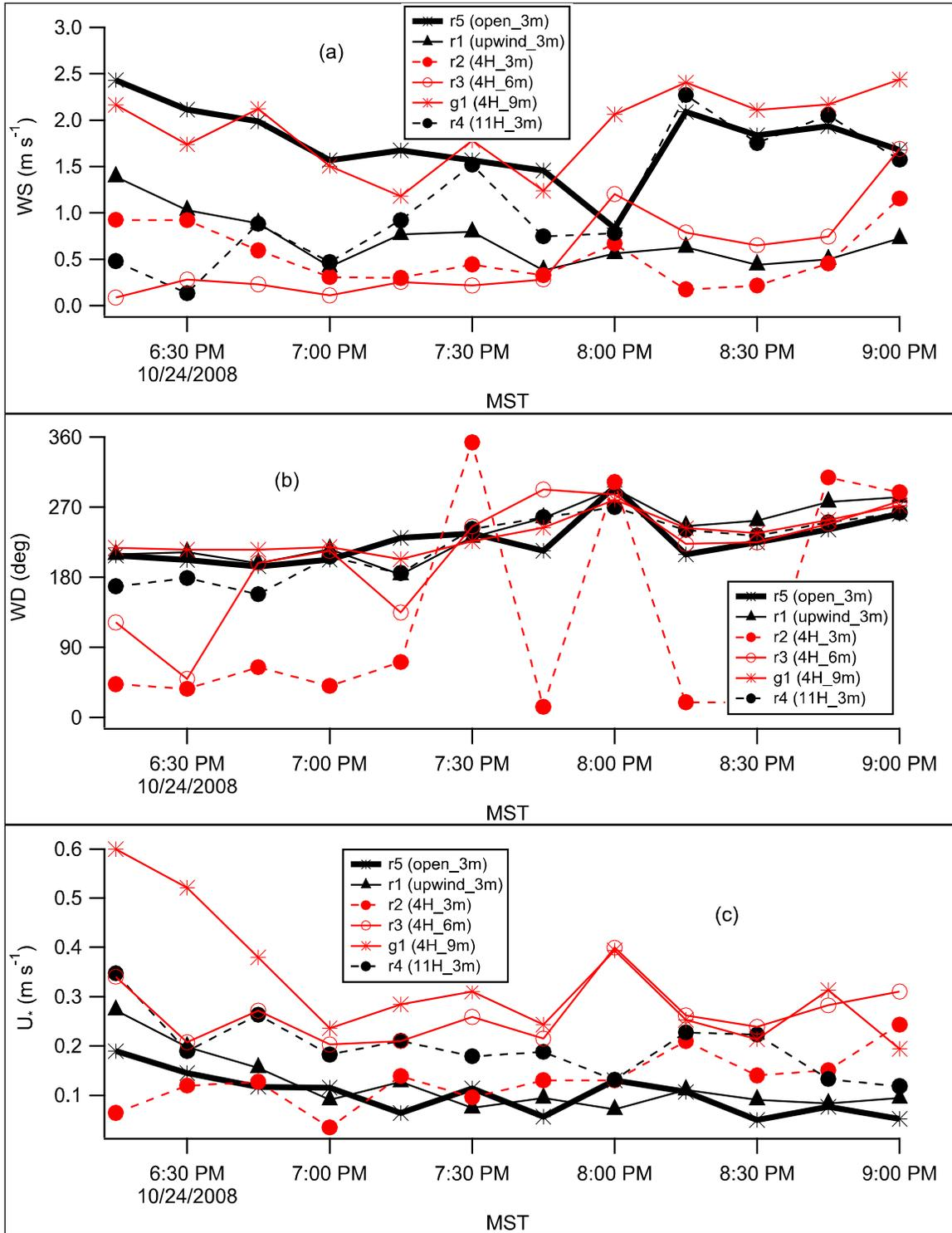
Figure 127. Test 5 sonic anemometer results for (a) wind speed, (b) wind direction, and (c) friction velocity  $u_*$ .
