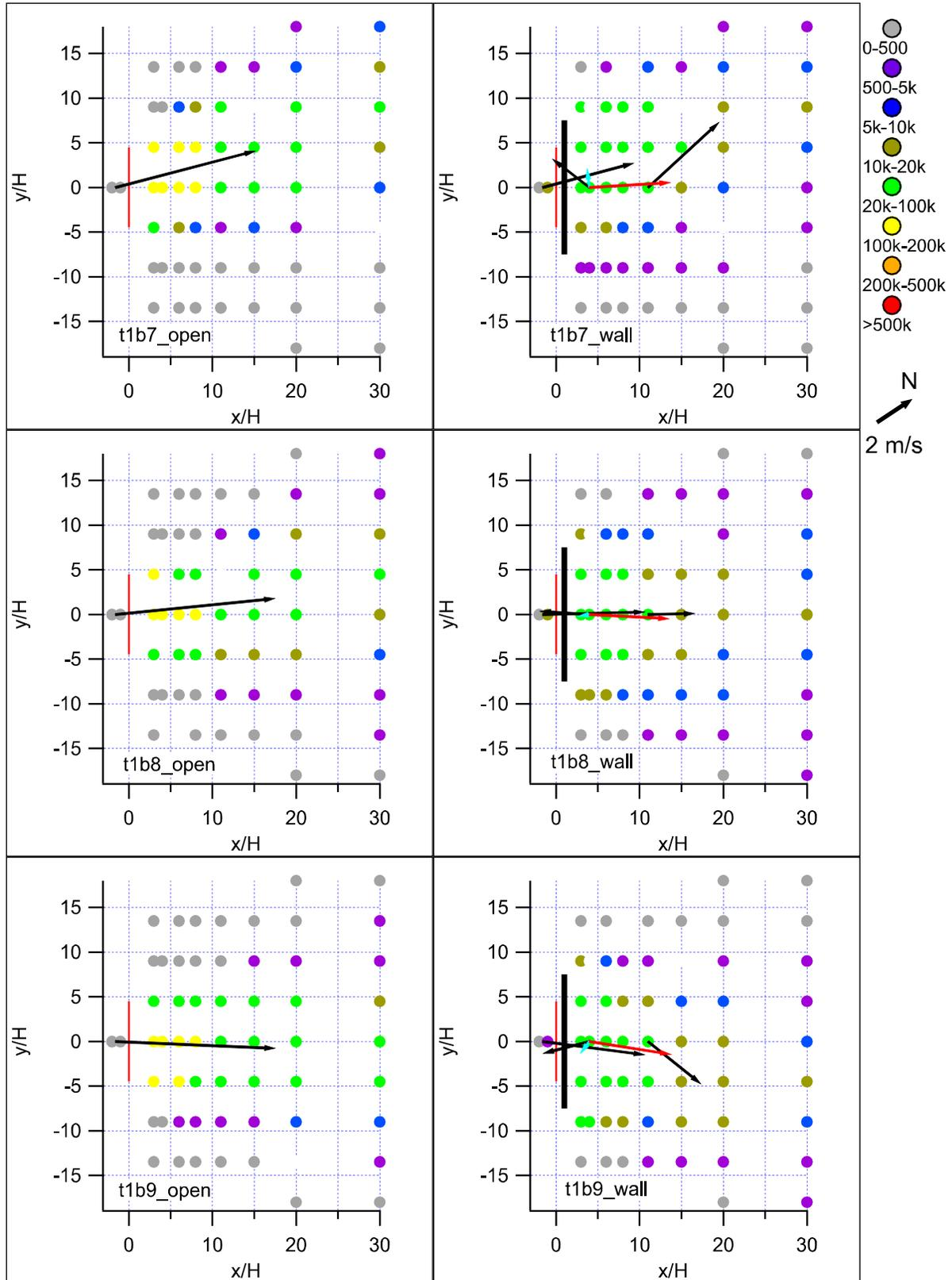
Figure 81. Normalized concentration/wind vector maps for Test 1, bags 7-9.
