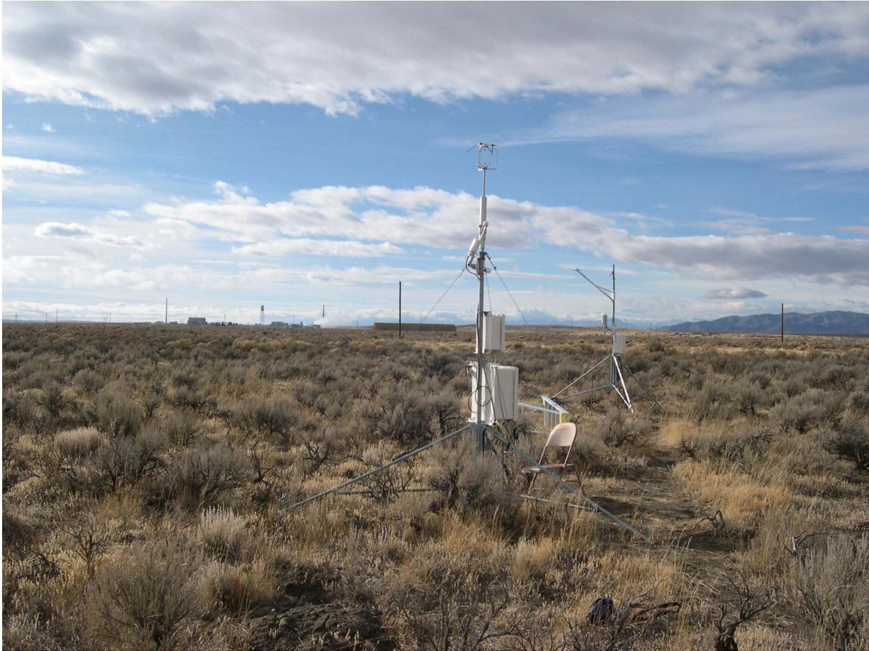
Figure 64. Two towers at Grid 3 that measure the energy flux.
