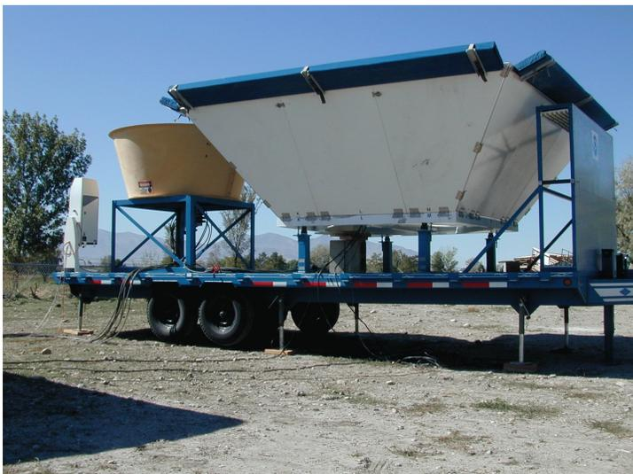
Figure 6. Doppler sodar and radar wind profiler.
