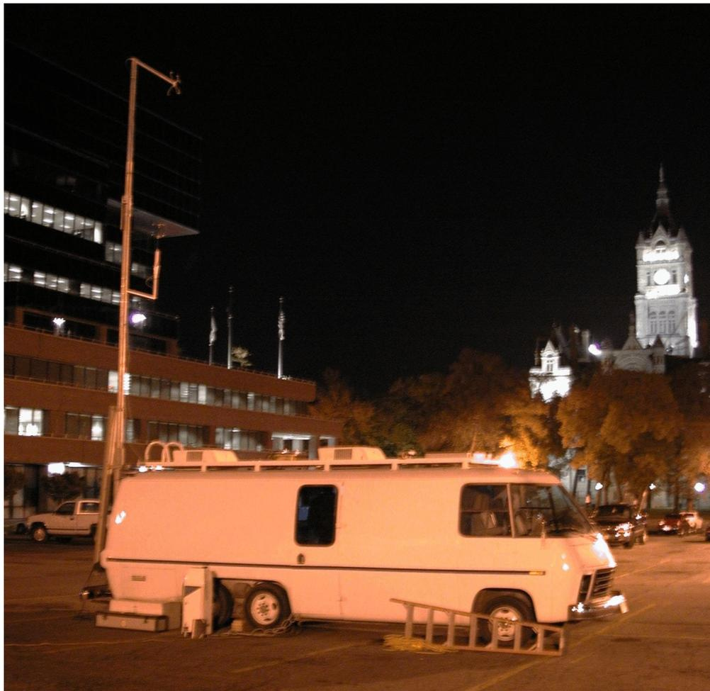
Figure 3. Sonic anemometers mounted on the LLNL mobile laboratory mast stationed in the City Centre (Chamber of Commerce) parking lot. The City Centre building can be seen to the left, while the City building tower can be seen at right. The tower is located across the street to the south of the parking lot.
