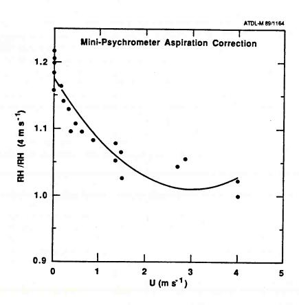
Correction coefficient for the Stitger and Welgraven (1976) minipsychrometers. These were developed empirically in a wind tunnel. Relative humidities are corrected to an aspiration velocity of 4 m s<sup>-1</sup>.
