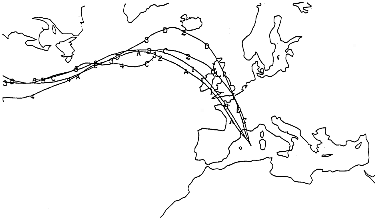
Figure 1. Example of 10-day back trajectories for January 7, 1981, from a point in the western Mediterranean. The 850-mb trajectories are A (00Z) and C (12Z); the 700-mb trajectories are B (00Z) and D (12Z). The numbers (1, 2, etc.) refer to days back in time.
