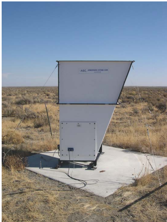
Figure 54. Photo of the ASC sodar, collocated with radar wind profiler at PRO.
