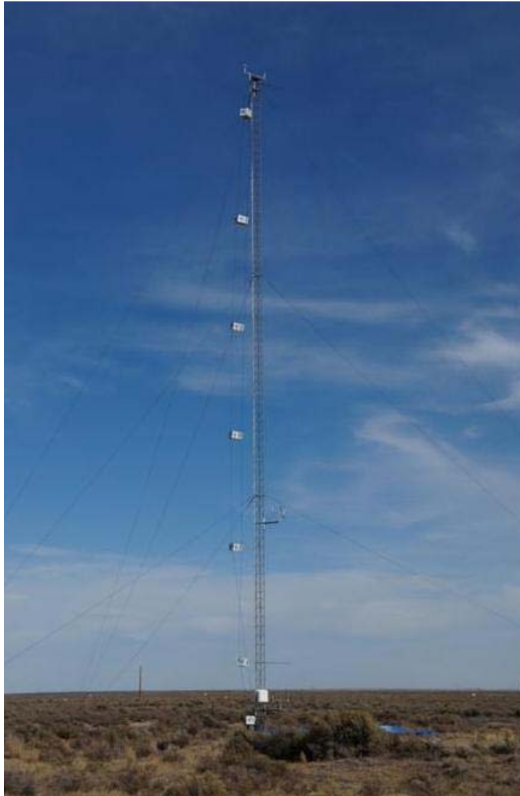
Figure 53. 30 m command center meteorological and tracer sampling tower (COC).
