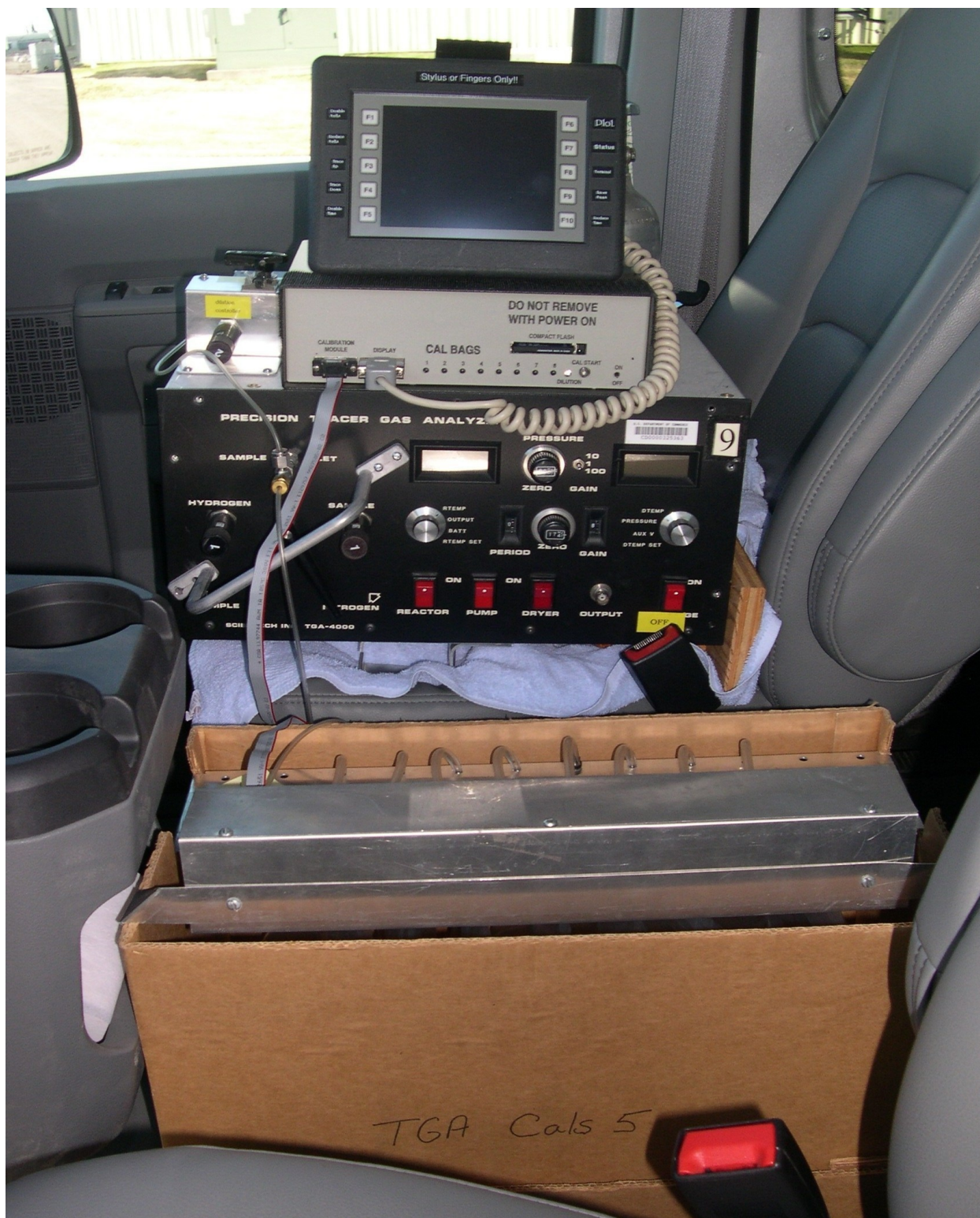
Figure 45. FRD mobile, fast response, tracer gas analyzer consisting of a data acquisition system, a TGA-4000 below the data acquisition system, and a calibration gas cartridge (foreground) installed in the passenger side seat.
