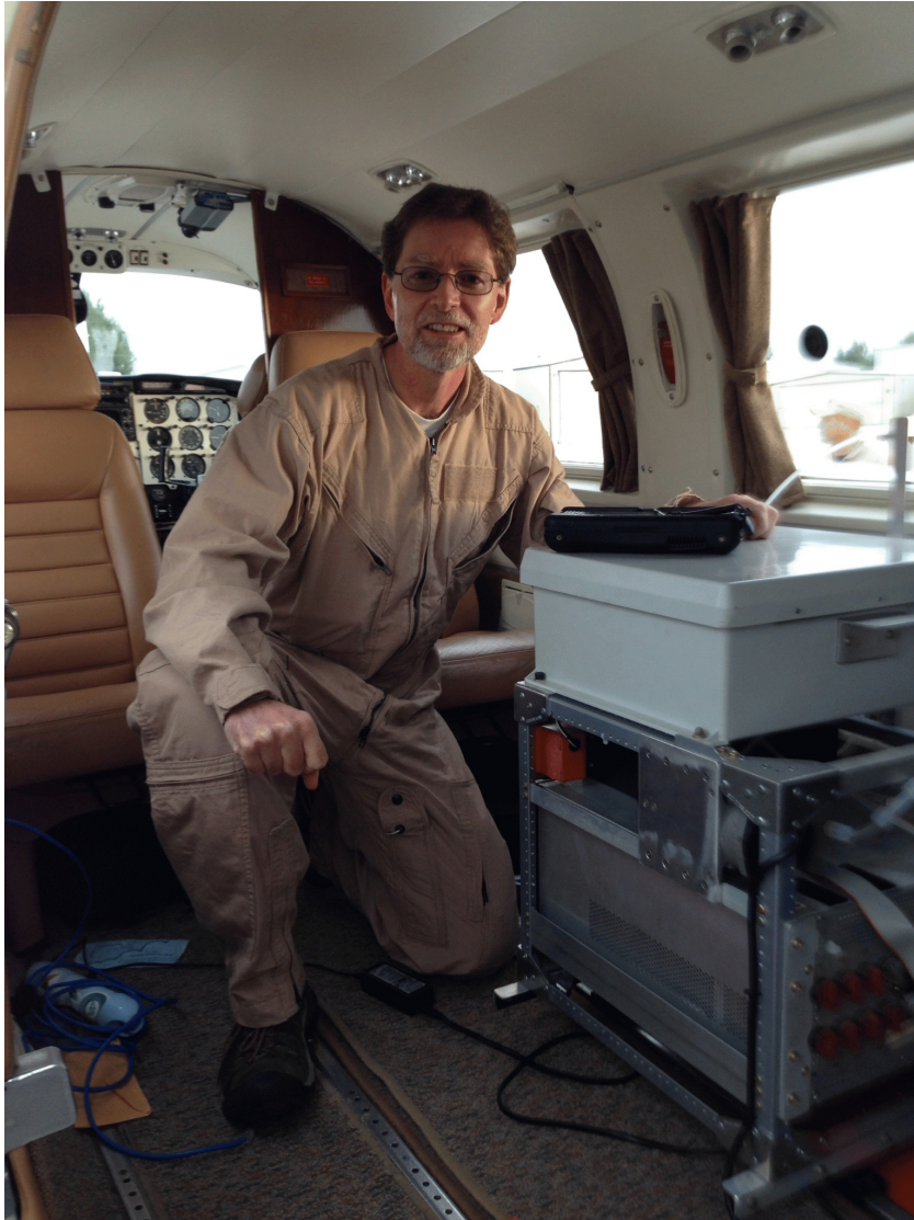
Figure 46. Fast response tracer gas analyzer system installed in Piper Navajo aircraft.
