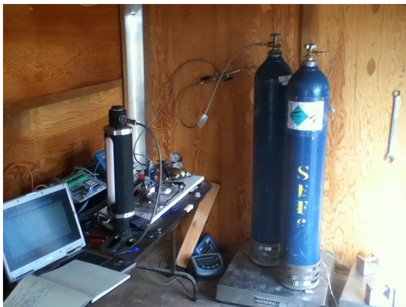
Figure 9. The SF 6 release system inside the cargo trailer including the SF 6 bottles, mass flow controller, computer data acquisition and control system, and electronic scales under the bottles.
