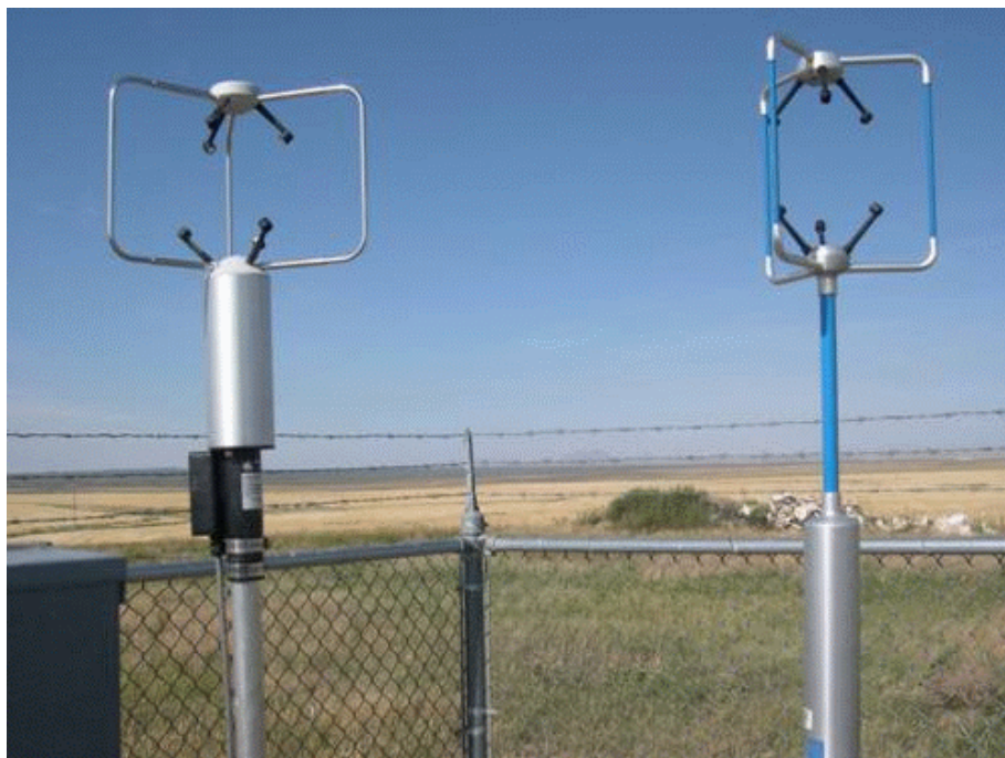
Figure 51. A closeup picture of an R. M. Young Ultrasonic 81000 (left) and a Gill Windmaster Pro (right) used during PSB1.
