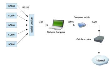
Figure 1: A diagram of the high frequency sonic anemometer data acquisition system
