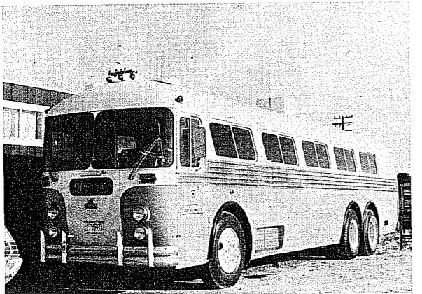
Figure 10. Mobile laboratory containing grid control and sample analysis equipment.
