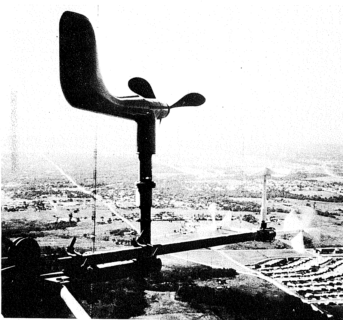
Figure 8. The orthogonal propeller anemometer in the extended position. At this time the propeller anemometer and the aerovane were being compared, normally the aerovane was removed to avoid interference.
