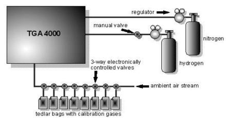
Figure 28. Schematic representation of the NOAA continuous  $SF_6$  tracer gas analyzer.
