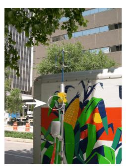
Figure 6. Point source dissemination from a tripod-mounted garden hose at 2 meters AGL. Sonic anemometer (top) and temp/ RH sensor (inside gray cylinder) is also attached to the tripod.
