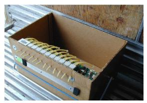
Figure 9. PIGS sampler box with the cartridge removed.
