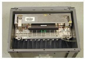
Figure 15. Super PIGS installed in a cartridge.
