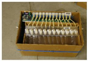
Figure 11. PIGS with sampler cartridge and D-cell battery (upper left) installed.
