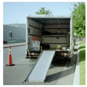
Figure 4. The  $SF_6$  release mechanism housed on a ledge inside the U-HAUL.
