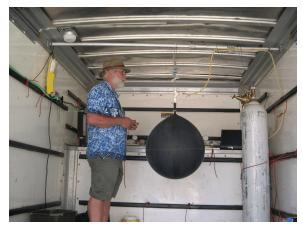
Figure 7. A meteorological balloon being filled with  $SF_6$  and weighed inside the U-haul in preparation for a puff release.
