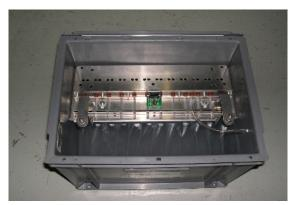
Figure 14. Super PIGS cartridge with sampler module removed.
