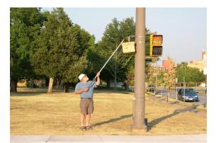
Figure 17. Sampler being hung on a utility pole.
