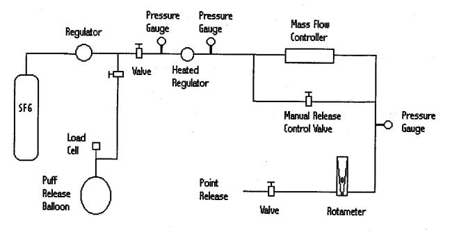
Figure 5. Schematic for both a puff and continuous point source SF<sub>6</sub> release mechanism.
