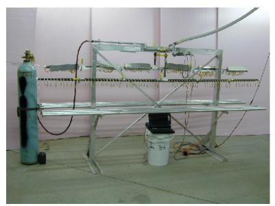
Figure A-1. Cartridge cleaning apparatus.
