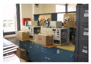
Figure 22. Two of the ATGAS in operation analyzing two PIGS cartridges.
