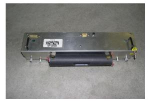
Figure 13. Super PIGS sampler module with black cylinder containing the 3 D-cell batteries.
