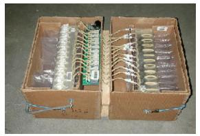
Figure A-7. PIGS control or blank sampler showing source cartridge (right) and receiver cartridge (left).
