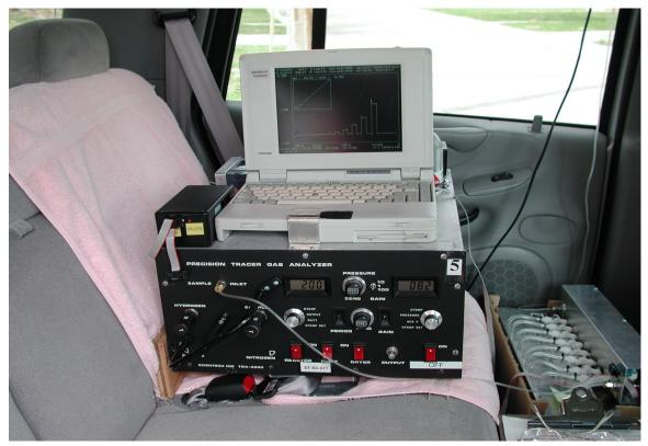
Figure 26. NOAA mobile tracer gas analyzer system, consisting of a laptop computer, a TGA-4000 below the laptop, and a calibration gas cartridge (lower right) installed in the rear seat of an SUV.
