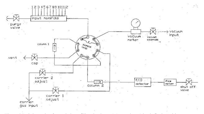
Figure 25. Schematic of sample loop fill and column 1 (pre-column) back-flush position.
