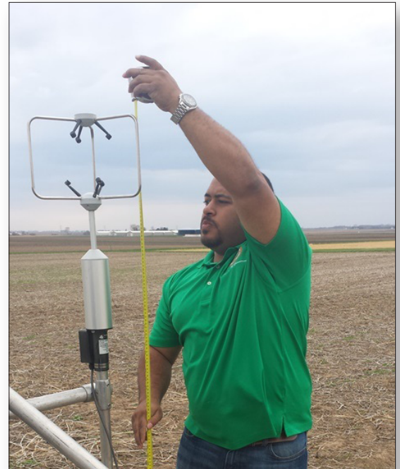
ATDD intern installing a sonic anemometer as part of a collaborative ammonia field study with the University of Illinois-Urbana Champaign at their Energy Biosciences Institute's Energy Farm in Urbana, IL. Photo: NOAA
