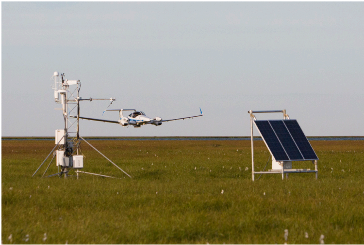
Aurora Flight Sciences Corporation's Centaur aircraft flies low over the ATDD flux measurement tower near Prudhoe Bay, Alaska. The aircraft carried a new airborne instrument system, designed by ATDD and Harvard University's Anderson Group, to measure fluxes of carbon dioxide and methane. These same compounds were measured by instruments on the tower to groundtruth the aircraft data. Photo credit: NOAA
