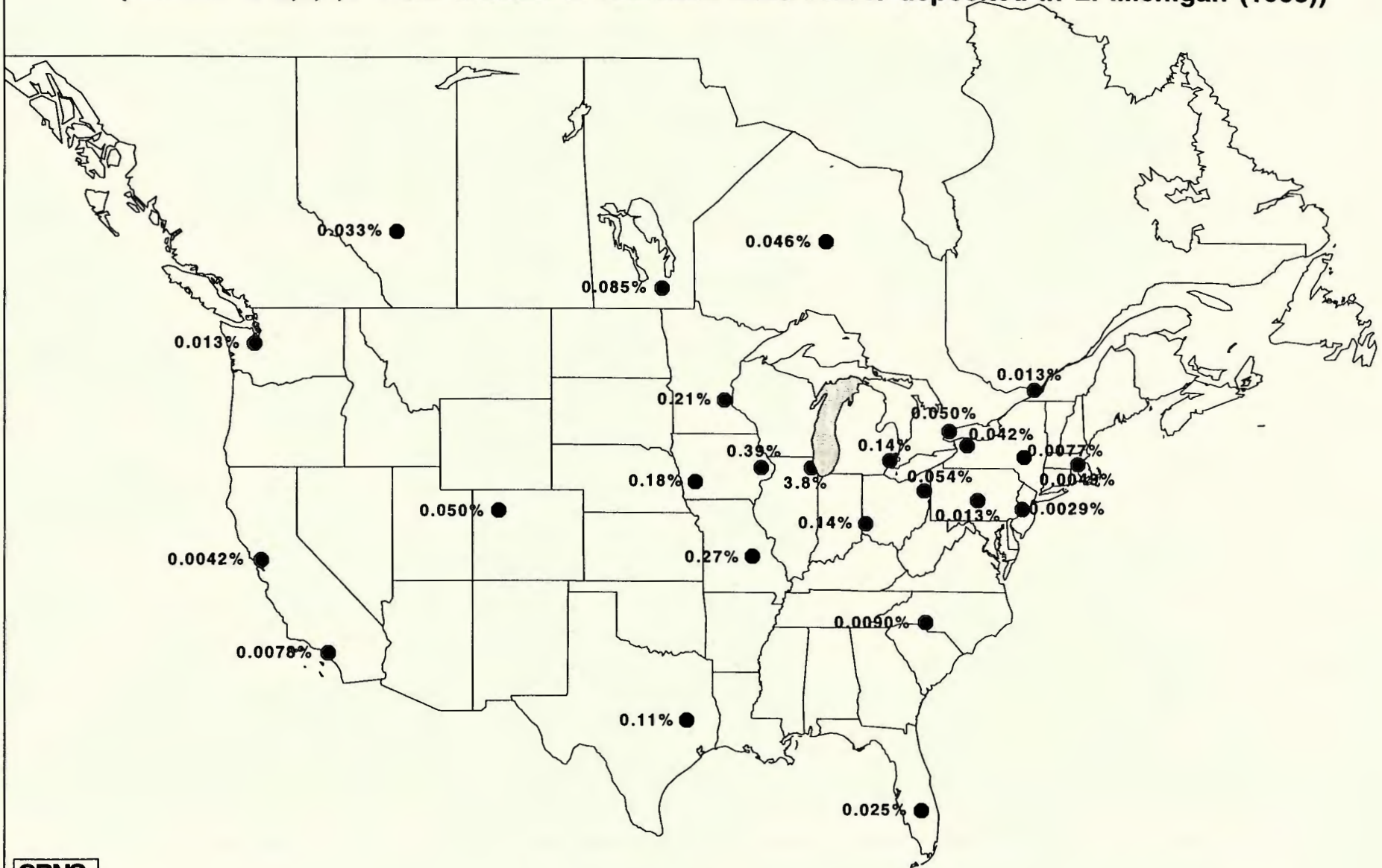
Fig. 3A: AIR TRANSFER COEFFICIENTS DIRECTLY COMPUTED BY THE MODIFIED HYSPLIT PROGRAM (Percent of 2,3,7,8-TCDD emitted at indicated sites that is deposited in L. Michigan (1993))
