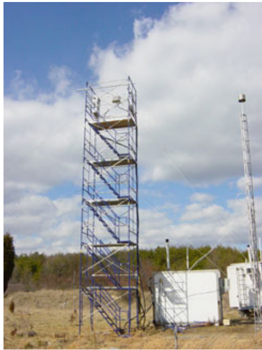
On left: A 10-meter high walk-up sampling tower at the Beltsville, Maryland site holds mercury instruments and meteorological sensors. On right: View of Tekran speciation system for the collection of fine particulate mercury (upper box) and reactive gaseous mercury (lower box)
