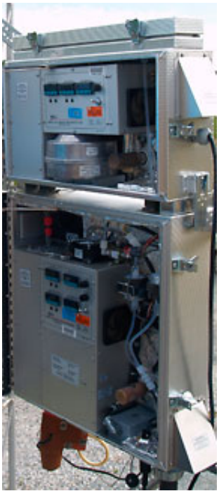
On left: A 10-meter high walk-up sampling tower at the Beltsville, Maryland site holds mercury instruments and meteorological sensors. On right: View of Tekran speciation system for the collection of fine particulate mercury (upper box) and reactive gaseous mercury (lower box)
