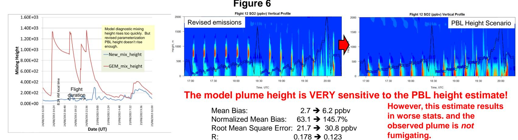
The plume rise algorithm is clearly very responsive to the PBL height parameterization used. This is worth investigating further, given the relatively poor performance of GEM's diagnostic PBL height estimate in the evening and early morning (Fig. 11, Brunner et al, 2015).
